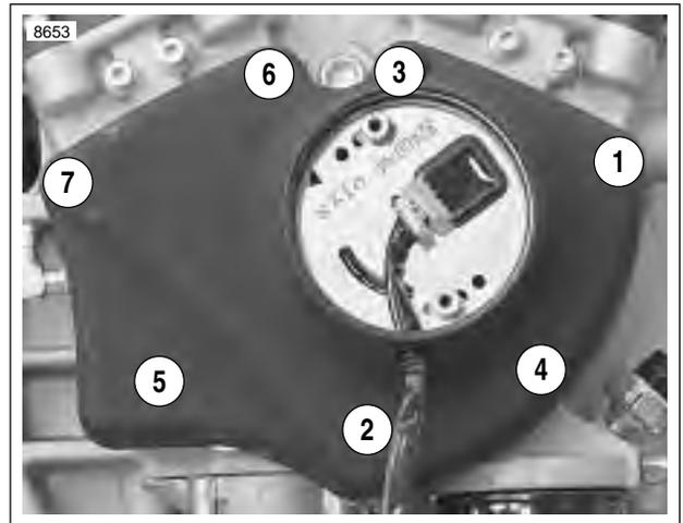
**Figure 3-129. Gearcase Cover Mounting Screw Torque Sequence**
