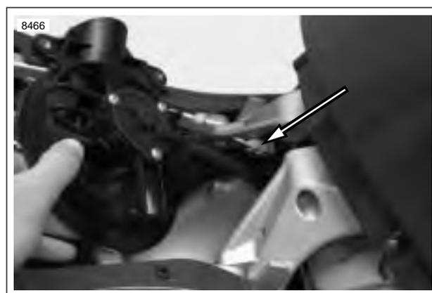
Figure 4-51. Cooling Fan Connector [97]
