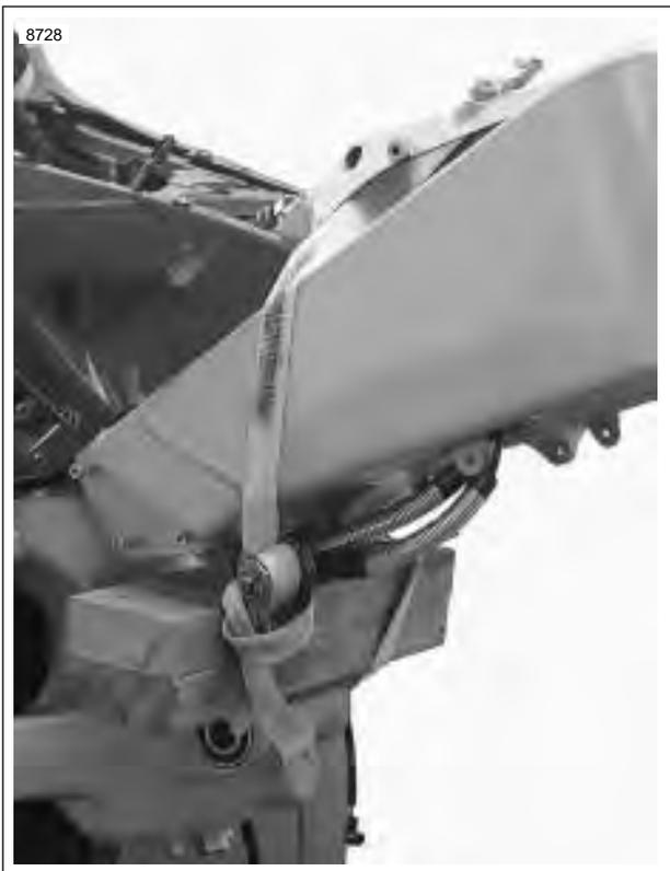
**Figure 3-32. Securing Vehicle for Relocation**
