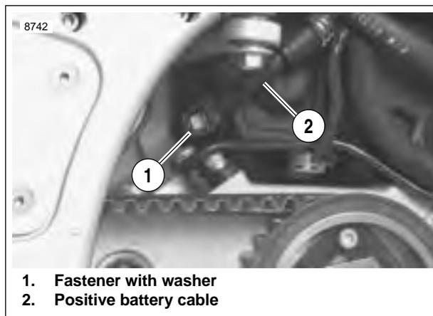
**Figure 7-40. Positive Battery Cable
