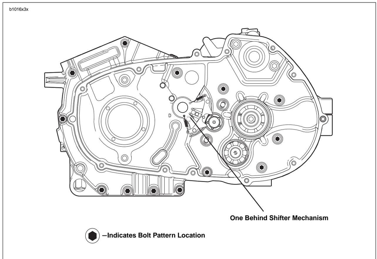
Figure 3-132. Crankcase Fasteners
