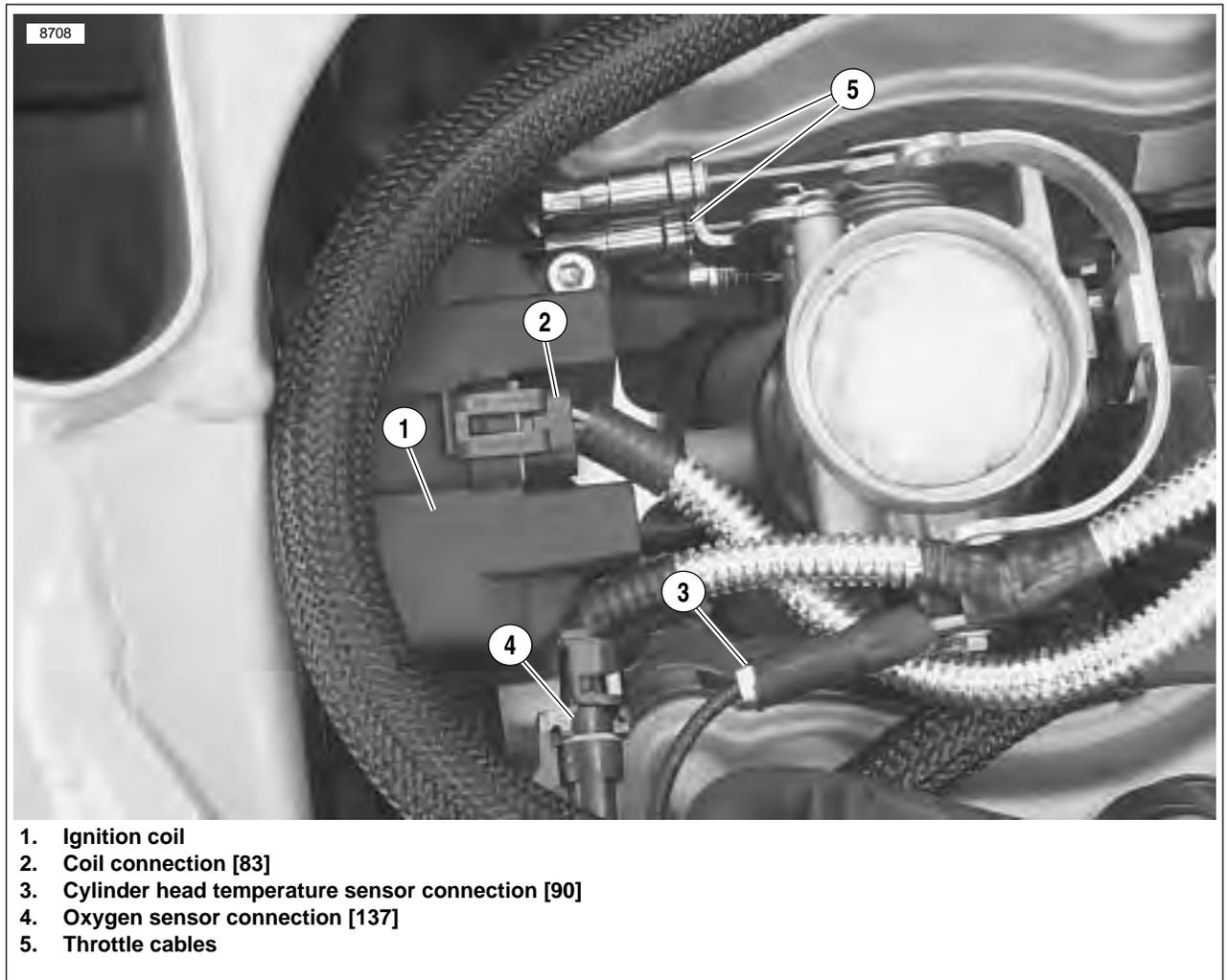
**Figure 3-2. Electrical Connections and Throttle Cables (Typical)**
