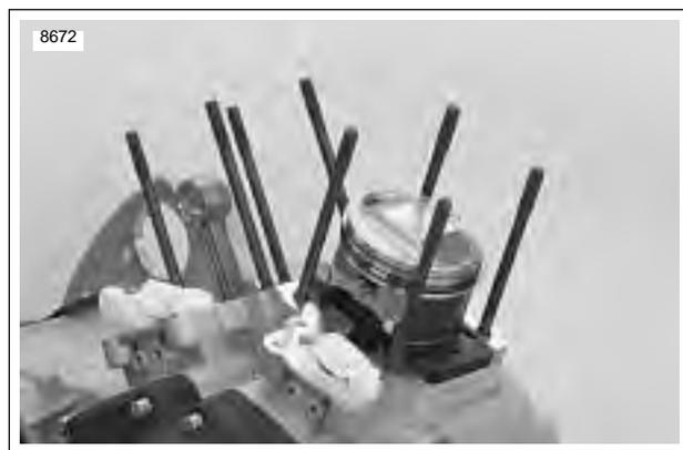
**Figure 3-108. Piston Support Plate**
