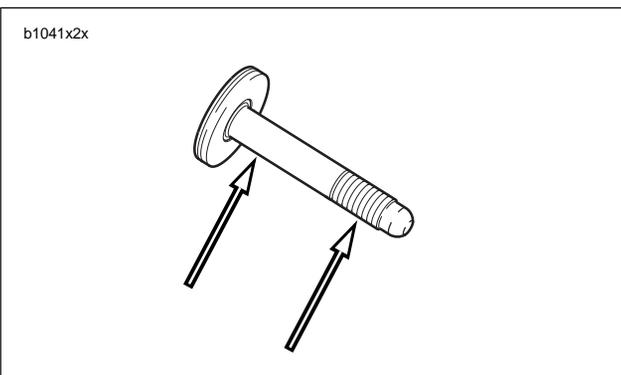
Figure 3-44. Lubrication Points on Front Isolator Bolt
