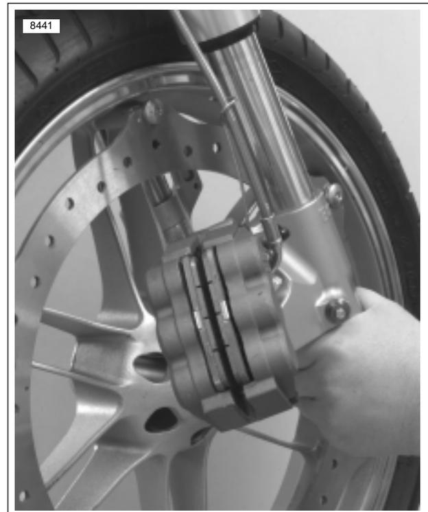
Figure 2-6. Front Wheel Removal and Installation
