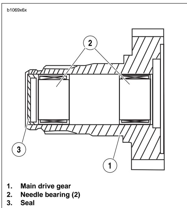
Figure 6-69. Main Drive Gear Assembly
