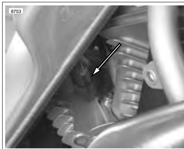
Figure 4-47. Throttle Position Sensor Location
