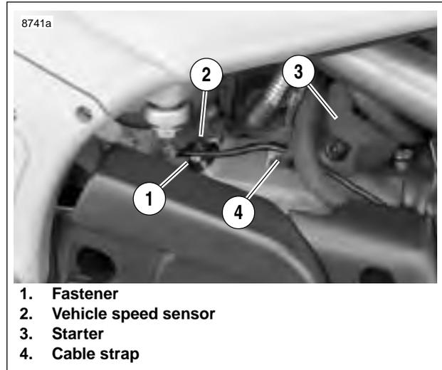
Figure 7-57. Speedometer Sensor
