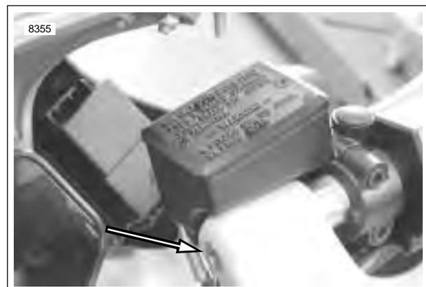
Figure 2-102. Handlebar Clip-on Mounting Fasteners (right clip-on shown)
