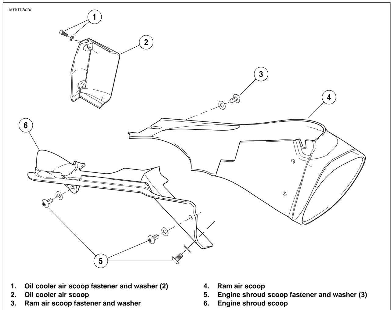
Figure 2-114. Ram Air Scoop, Engine Shroud, Oil Cooler
