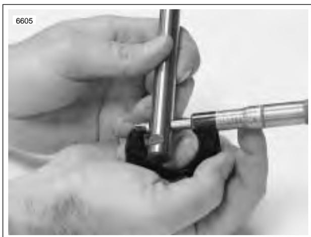
**Figure 3-68. Measuring Rocker Arm Shaft Diameter (Rocker Arm Bushing Position)**
