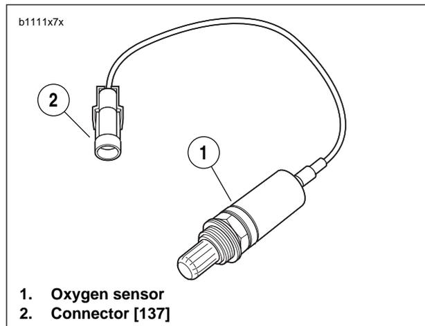
Figure 4-34. Oxygen Sensor
