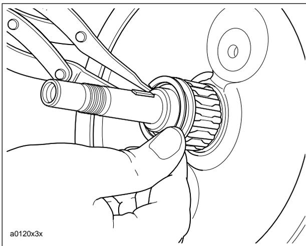
**Figure 3-151. Pinion Shaft Bearing**
