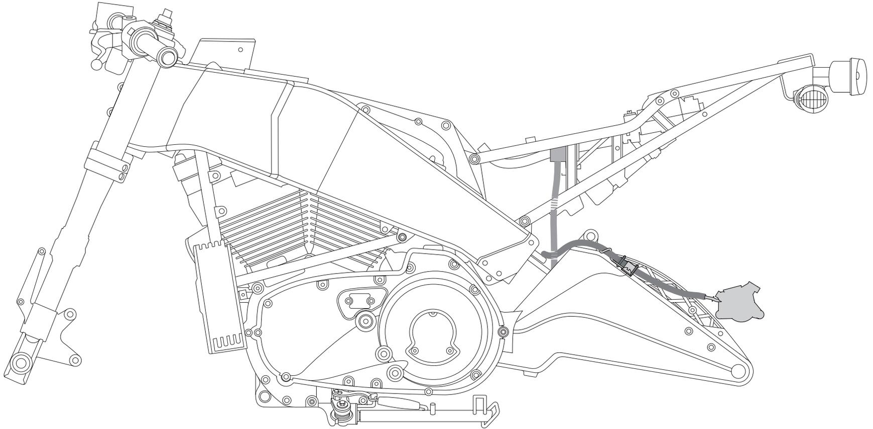
Figure D-3. Rear Brake Systems, Left Side View
