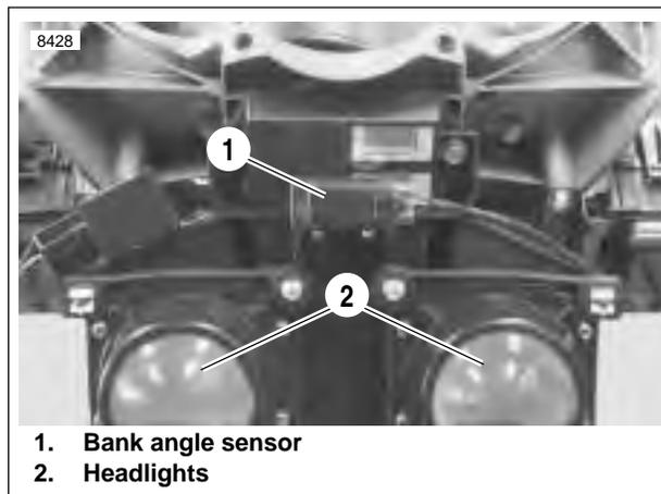
Figure 4-45. Bank Angle Sensor
