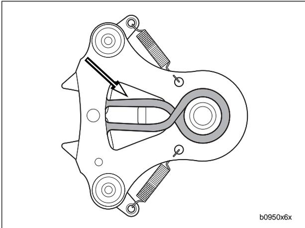
**Figure 6-90. Shifter Shaft Return Spring
