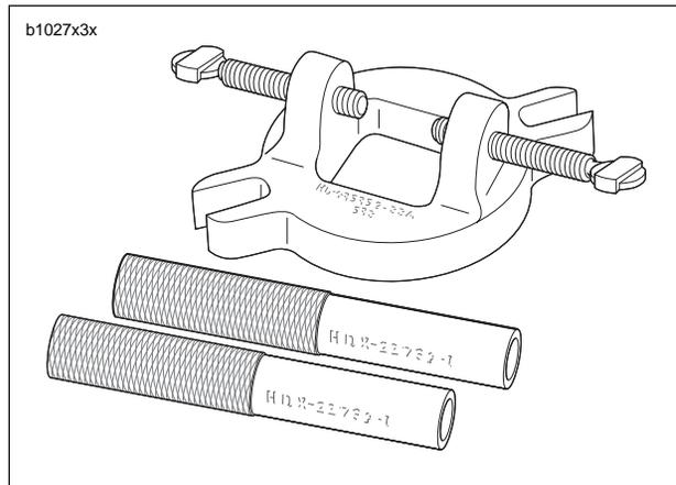
**Figure 3-100. Connecting Rod Clamping Tool (Part No. HD-95952-33B)**
