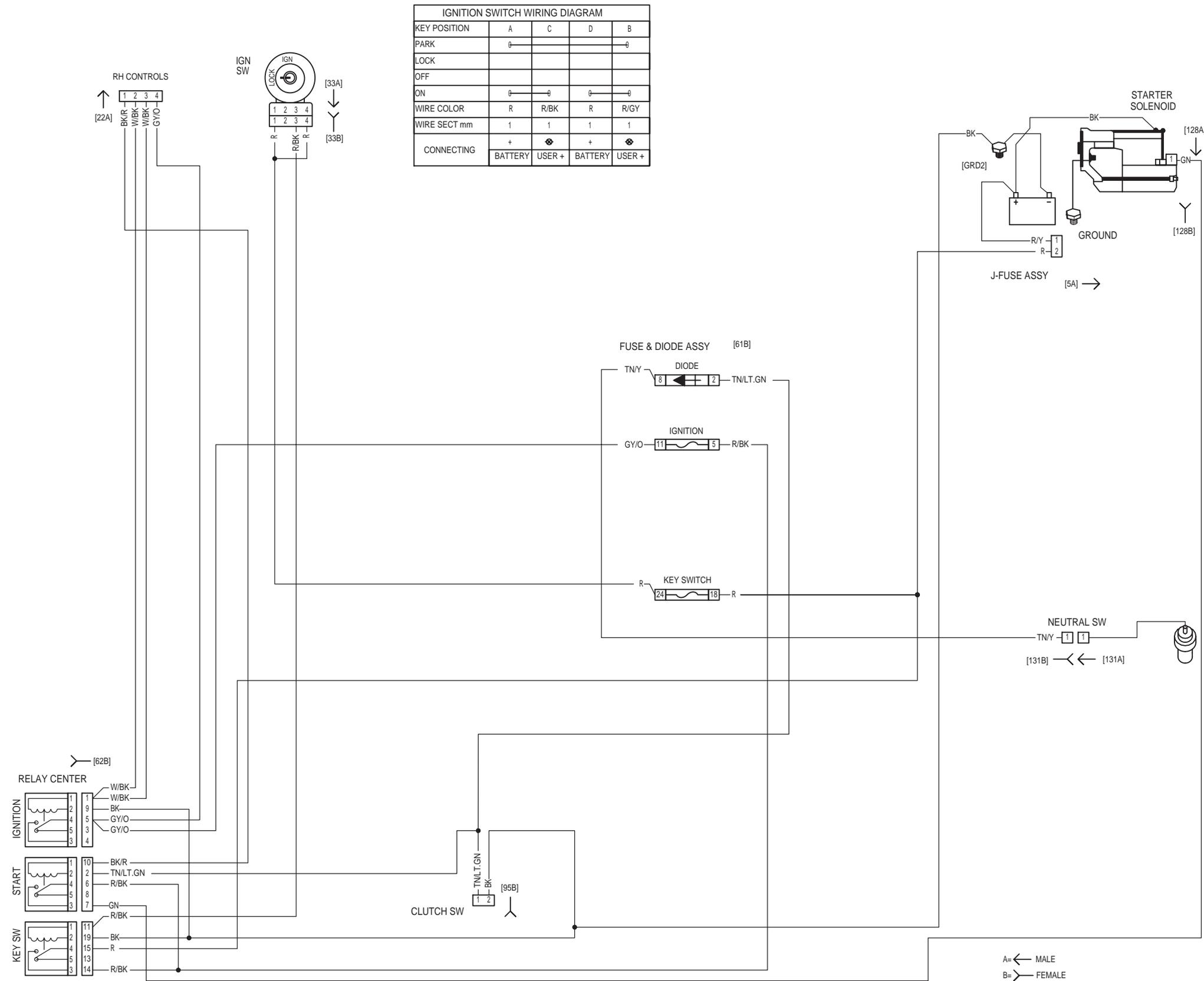
**IGNITION SWITCH WIRING DIAGRAM**
