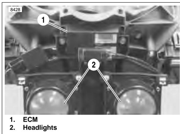
Figure 4-17. Electronic Control Module
