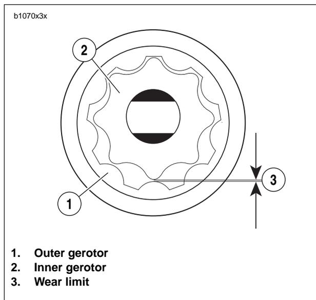
Figure 3-118. Gerotor Wear Limits
