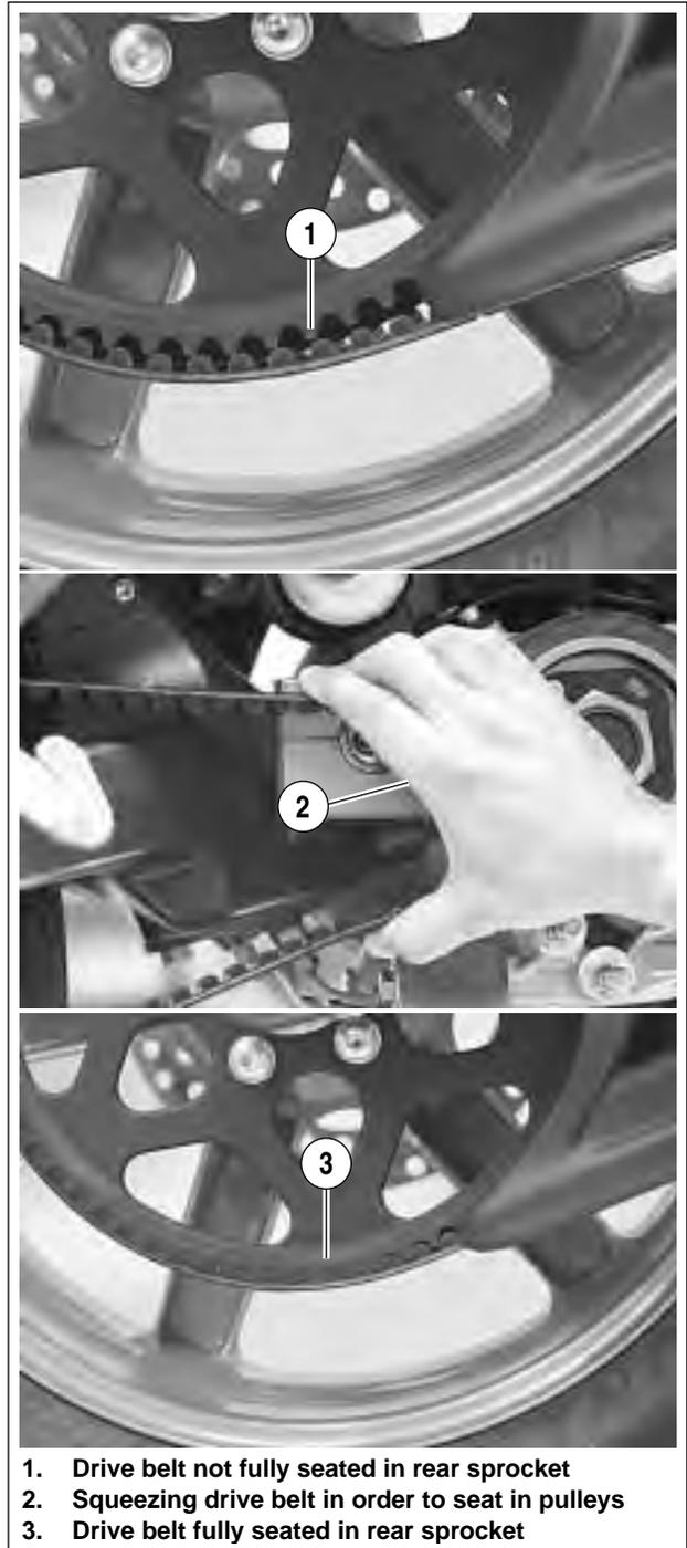
1. Drive belt not fully seated in rear sprocket
