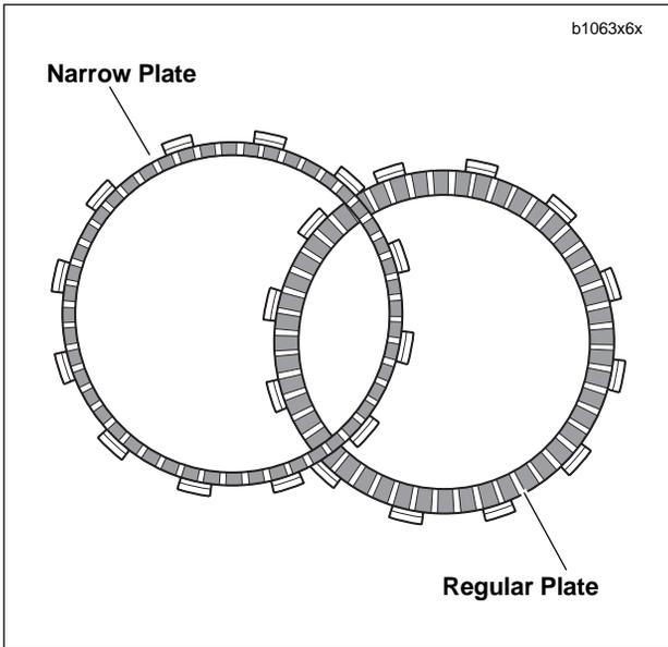
Figure 6-18. Friction Plates
