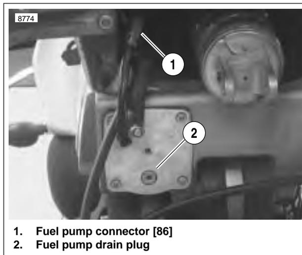
**Figure 4-64. Fuel Pump Drain Screw (swingarm removed for illustration)**
