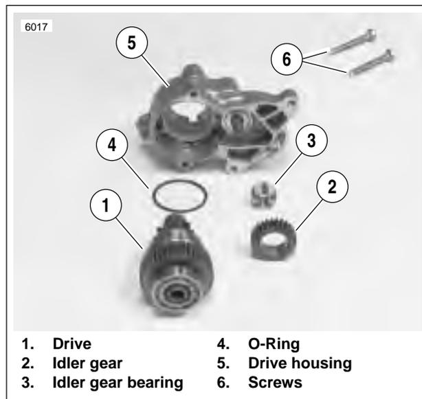
Figure 5-24. Starter Drive Assembly
