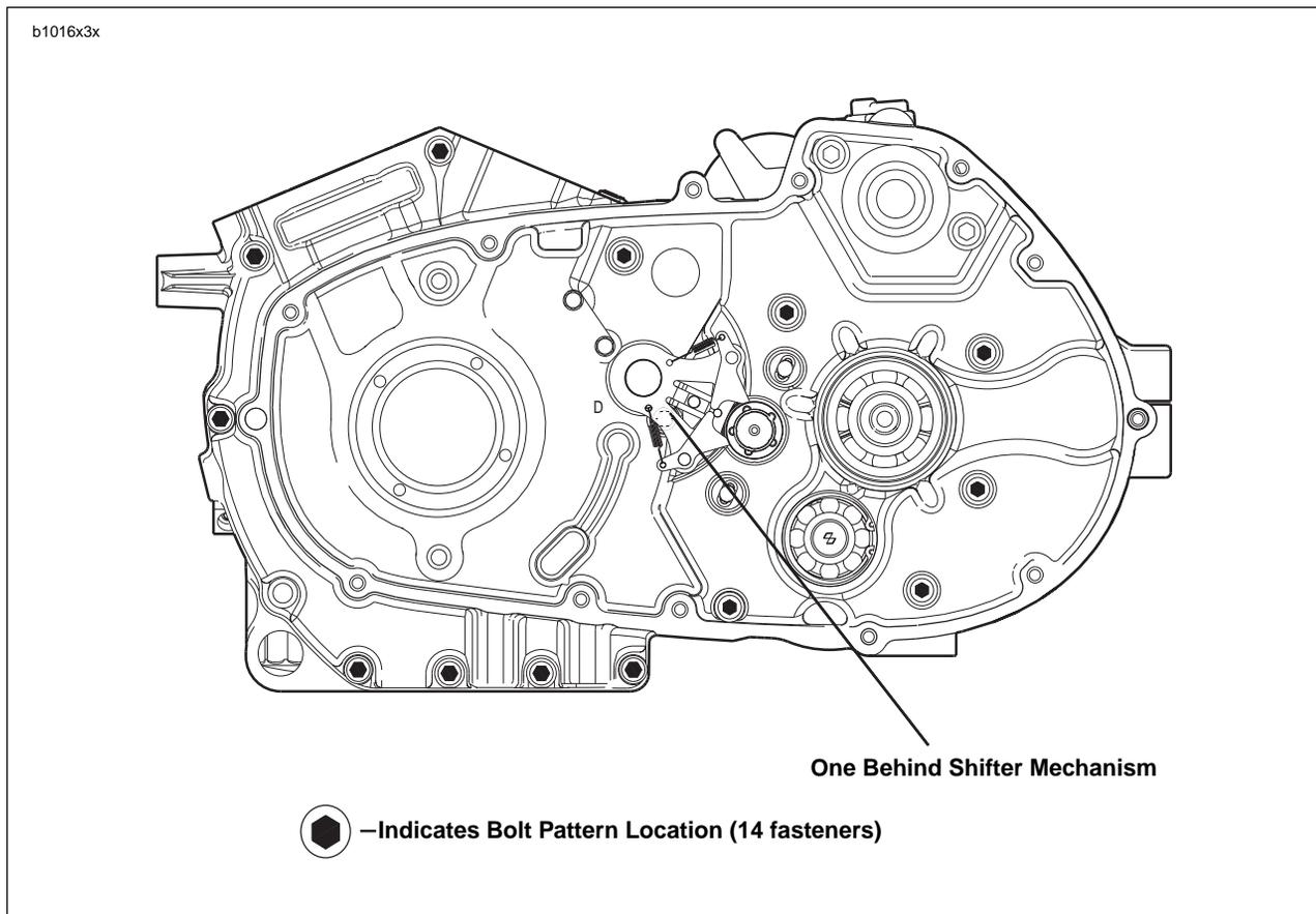
Figure 6-53. Crankcase Fasteners
