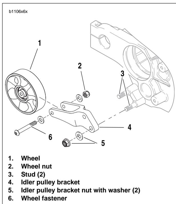
Figure 6-94. Idler Pulley Assembly
