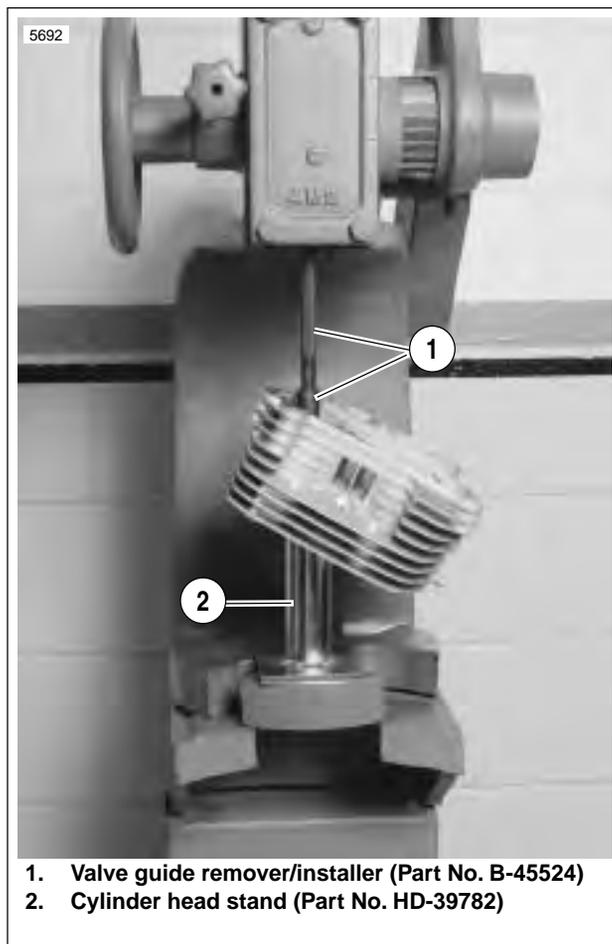
1. Valve guide remover/installer (Part No. B-45524)
