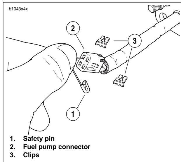
Figure 4-59. Fuel Pump Connector Disassembly
