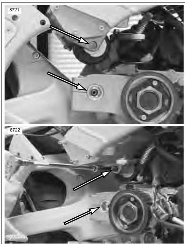
**Figure 3-25. Rear Isolator Bolt and Swingarm Pivot Shaft**
