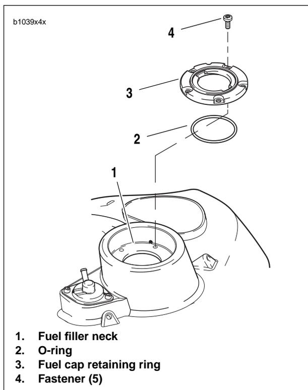
**Figure 4-65. Fuel Cap Retaining Ring**
