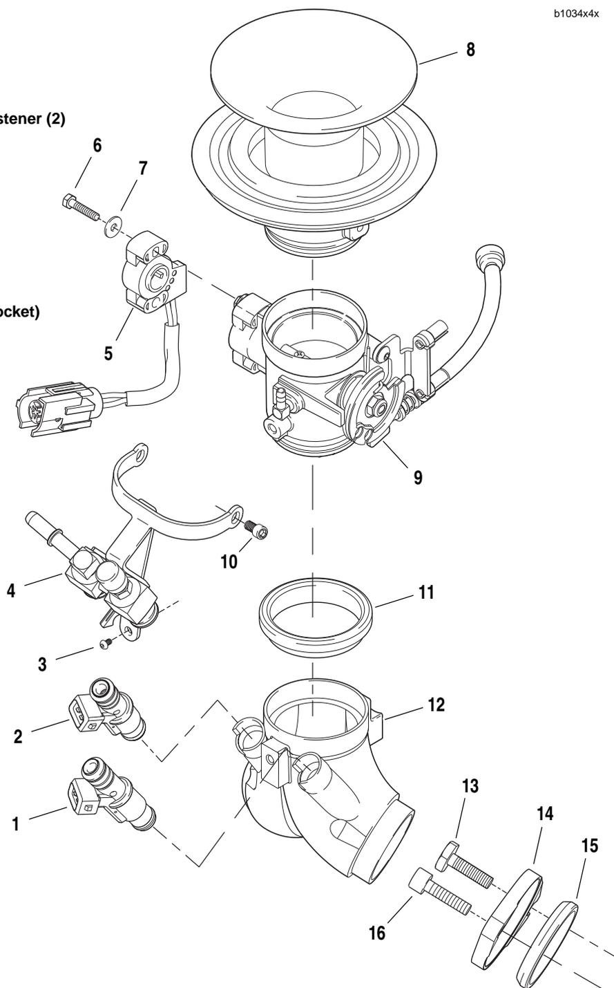
Figure 4-67. Throttle Body/Intake Manifold Assembly
