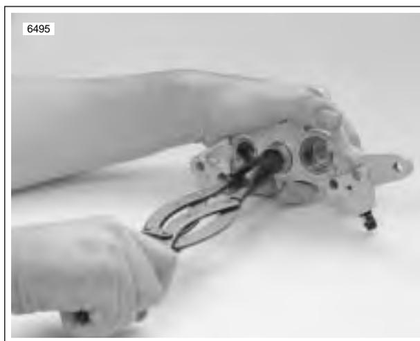
Figure 2-46. Removing Pistons (B-42887)
