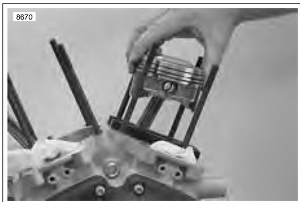
**Figure 3-104. Piston Support Plate**
