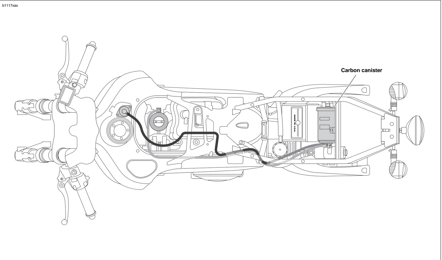
Figure D-4. Evaporative Emissions Control, California Models, Top View
