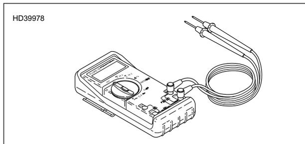
**Figure 4-11. Fluke 78 Multimeter (DVOM)
