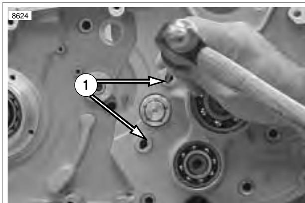
1. Slots for removing the shifter fork shafts
