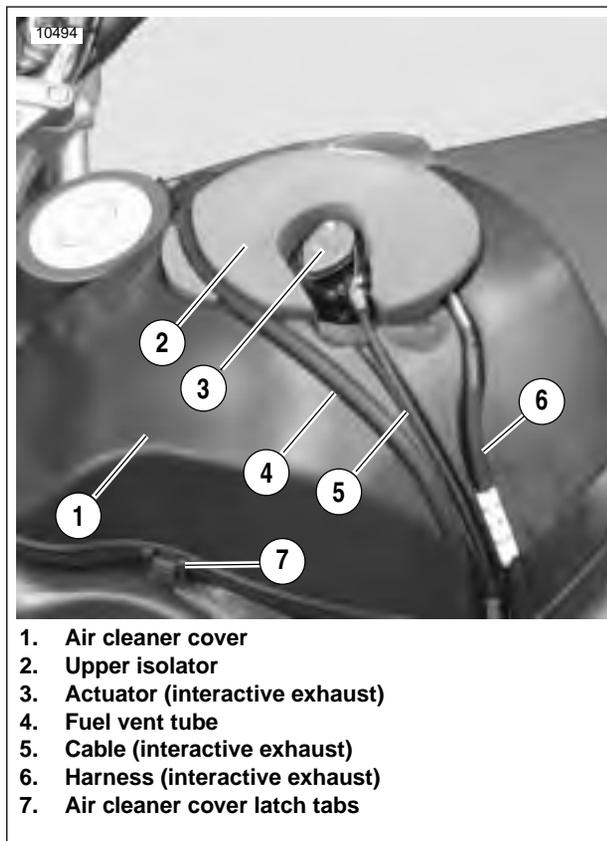
Figure 1-38. Air Cleaner Cover, Fuel Vent Tube and Fuel Vapor Valve (XB12)
