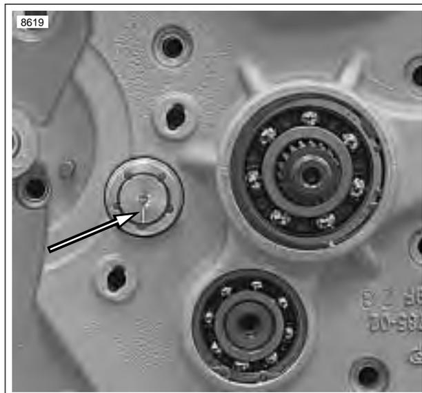
**Figure 6-88. Scribed Line on Shifter Drum at 6 O'clock (Transmission in 4th Gear)**
