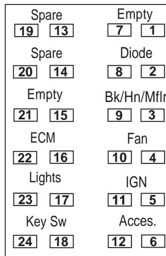
Figure 4-43. Fuses and Diode
