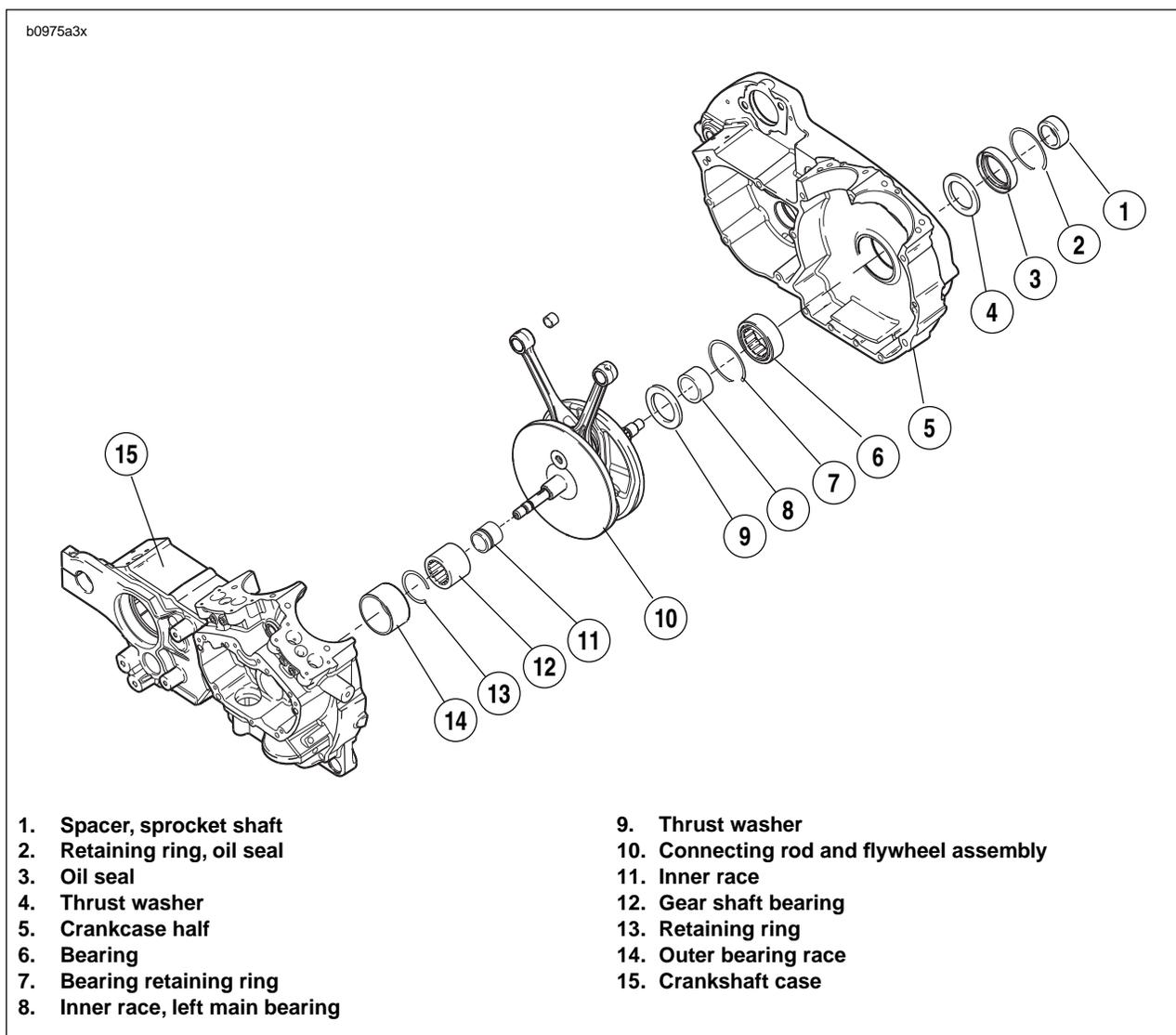
**Figure 3-135. Crankcase and Flywheel Assembly**
