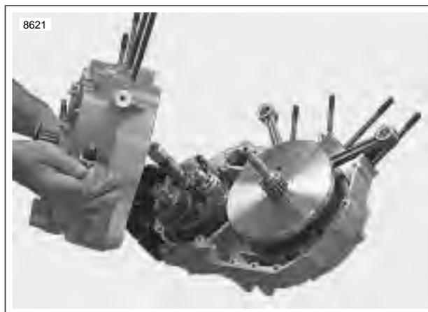
**Figure 6-89. Crankcase Halves**
