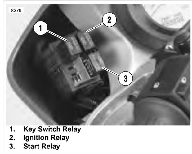
Figure 4-39. Electrical Relays
