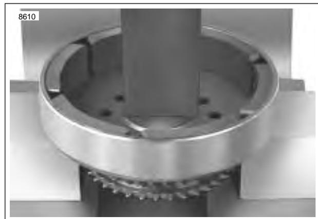
Figure 7-33. Removing Rotor From Sprocket
