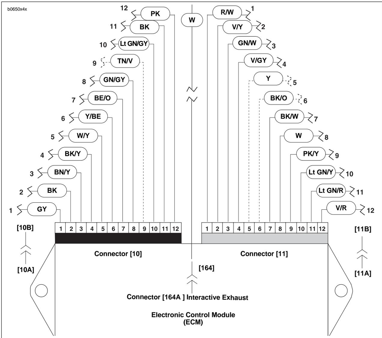
Figure 4-32. ECM Wiring (Interactive Muffler Connector [164] XB12R Only)
