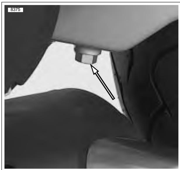
Figure 1-4. Oil Tank Drain Plug
