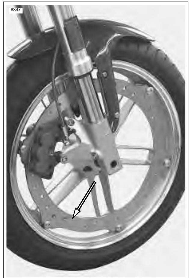
Figure 1-14. Front Brake Rotor
