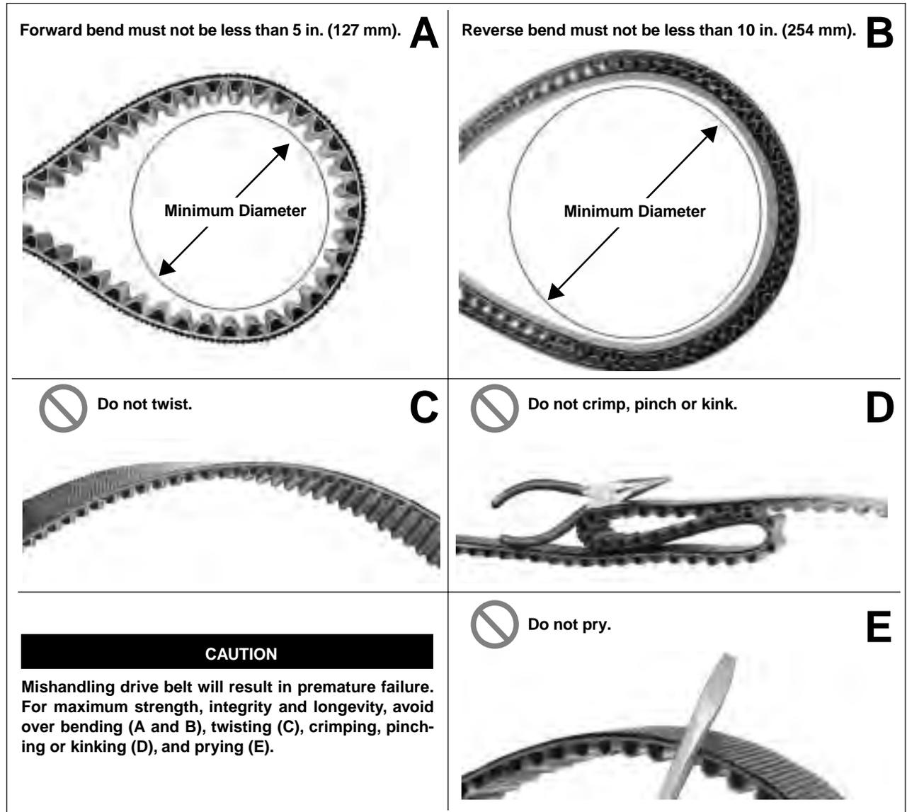
Figure 6-37. Proper Drive Belt Handling
