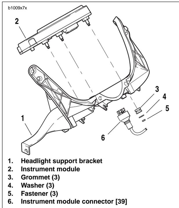
Figure 7-62. Instrument Module
