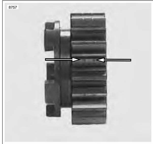
**Figure 6-66. New Mainshaft 1st Gear with Identification Grooves**
