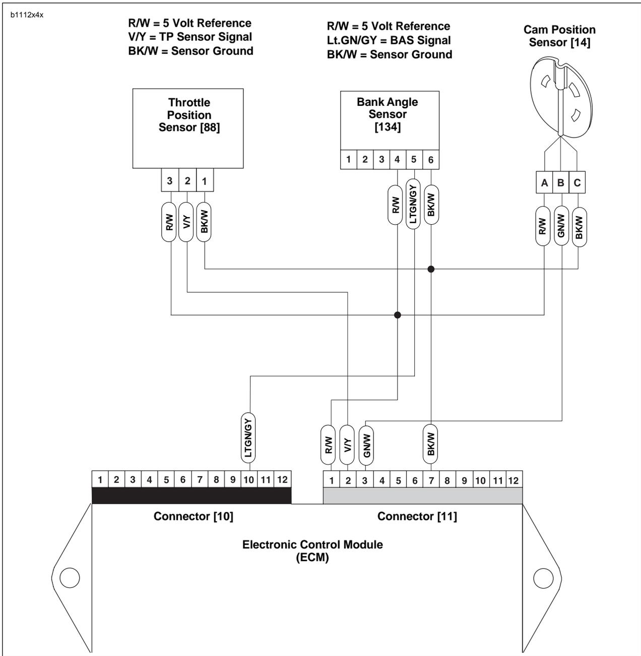
Figure 4-62. Cam Position Sensor Circuit
