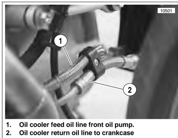
Figure 3-52. Oil Cooler Oil Lines
