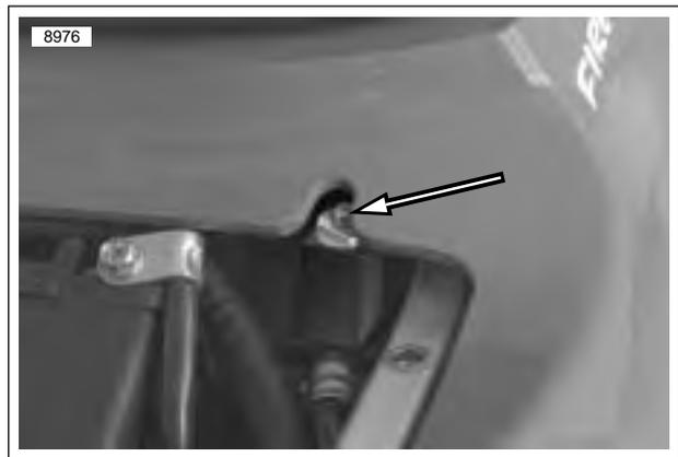
**Figure 1-34. Rear Shock Compression Adjustment**
