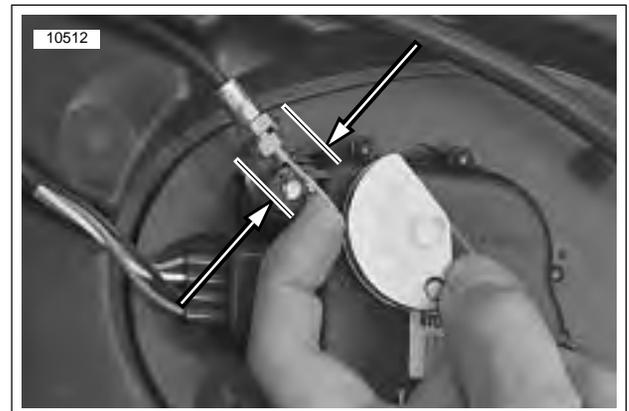
Figure 1-45. Checking For 1/8 in. (3.18) Maximum Free Play In Either Direction For Proper Adjustment
