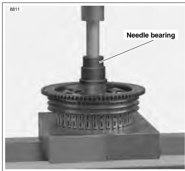
Figure 6-31. Installing Clutch Shell Needle Bearing Clutch Shell Bearing Remover/Installer B-45926
