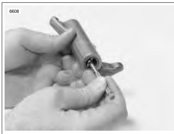
**Figure 3-70. Measuring Rocker Arm Bushing Inner Diameter**
