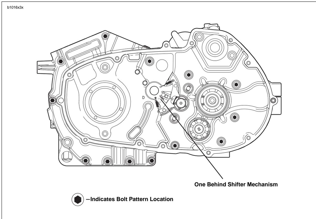
**Figure 3-152. Crankcase Fasteners**
