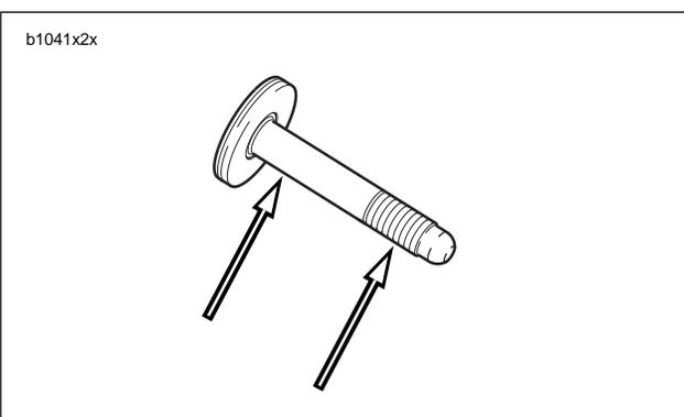
**Figure 3-9. Lubrication Points on Front Isolator Bolt**
