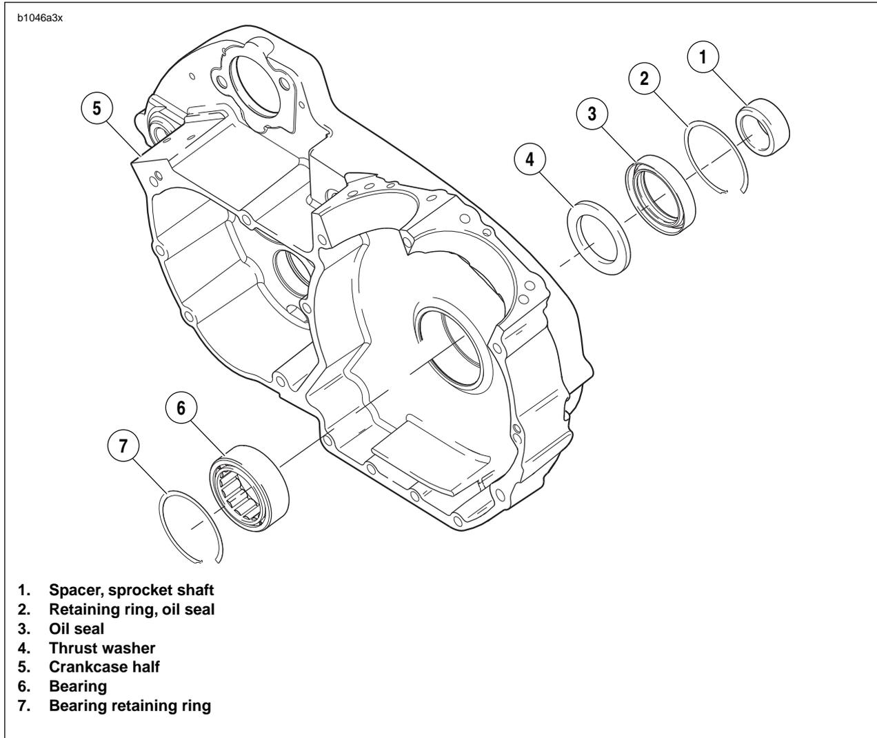
Figure 3-148. Left Main Bearing Assembly
