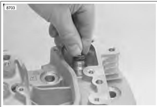
**Figure 3-81. Valve Seal and Lower Collar Assembly Installation**
