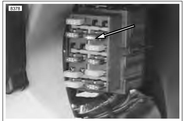
**Figure 7-17. Fuse Block (contains diode)**
