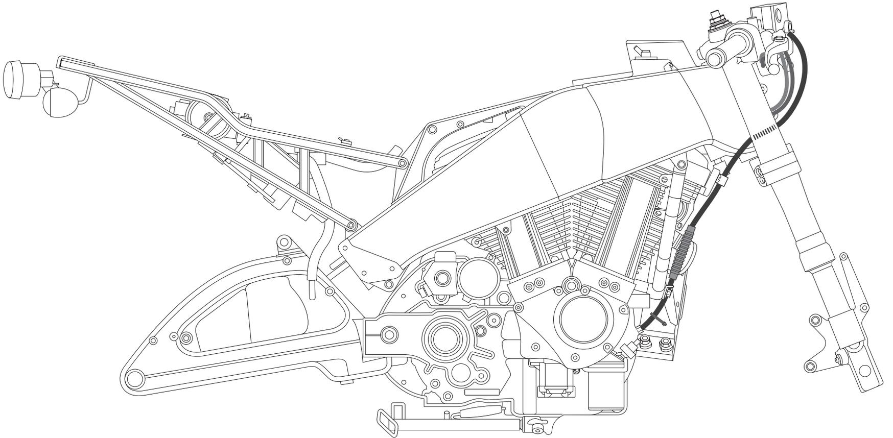
Figure D-11. Clutch and Throttle Cables, Right Side View
