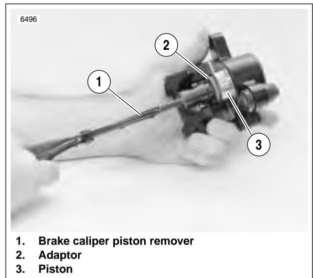
1. Brake caliper piston remover
