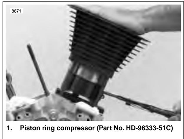
**Figure 3-109. Compressing Piston Rings**
