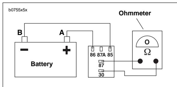
**Figure 7-16. Starter Relay Test**
