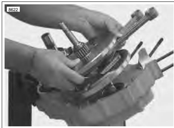
**Figure 3-134. Removing Flywheels from Left Crankcase**
