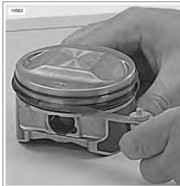
**Figure 3-99. Measuring Ring Clearance in Groove**
