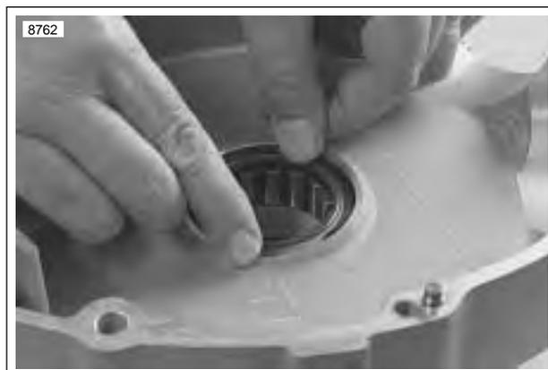
**Figure 3-138. Removing Left Main Bearing Retaining Ring**
