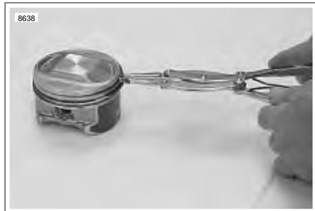
**Figure 3-92. Removing Piston Rings**
