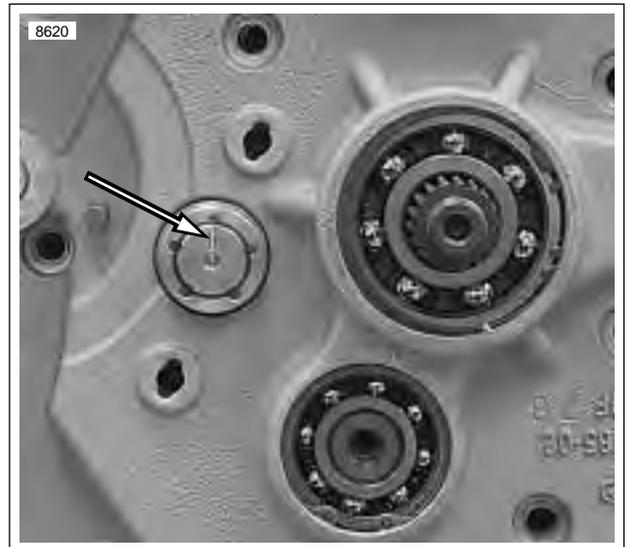
**Figure 6-51. Scribed Line on Shifter Drum at 12 o'clock (Transmission in Neutral)**
