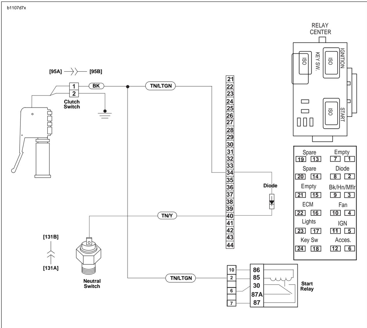
Figure 7-13. Diode Wiring
