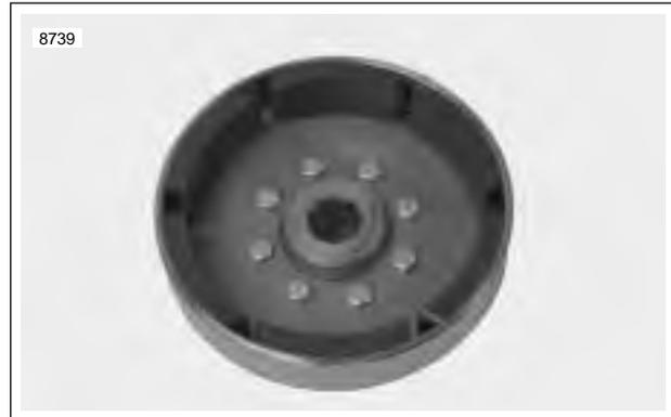
Figure 7-32. Rotor Assembly
