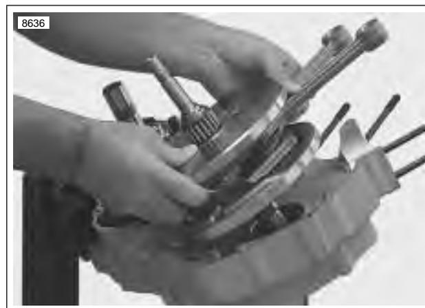
Figure 6-55. Removing Flywheels from Left Case Half
