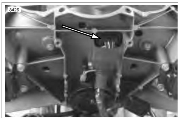
Figure 4-54. Instrument Module Connector [39]
