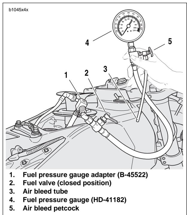
Figure 4-26. Fuel Pressure Gauge (Part No. HD-41182)
