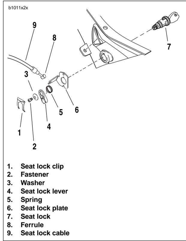
Figure 2-123. Seat Lock and Cable Assembly
