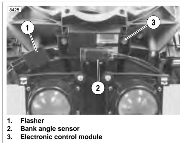
Figure 2-97. Headlight Support Bracket
