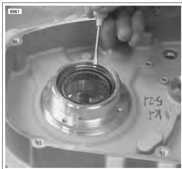
**Figure 3-137. Left Main Seal Retaining Ring**
