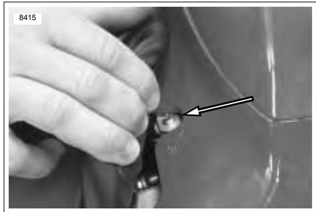
**Figure 1-33. Accessing Rear Shock Compression Adjuster**
