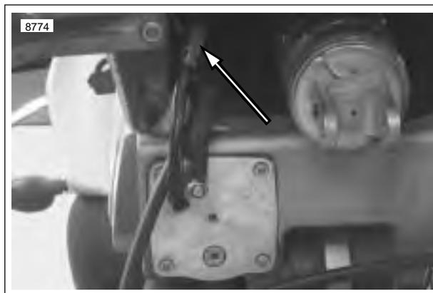
Figure 4-23. Fuel Pump Connector [86] (swingarm removed for illustration)
