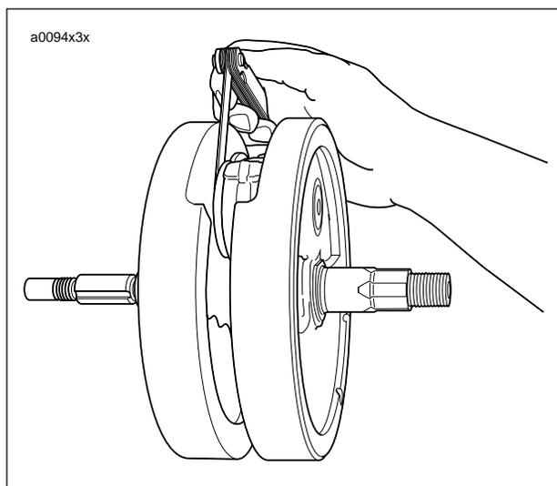
**Figure 3-147. Checking Connecting Rod Side Play**
