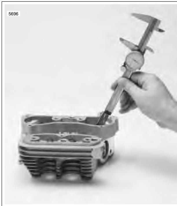
Figure 3-71. Measuring Valve Stem Protrusion
