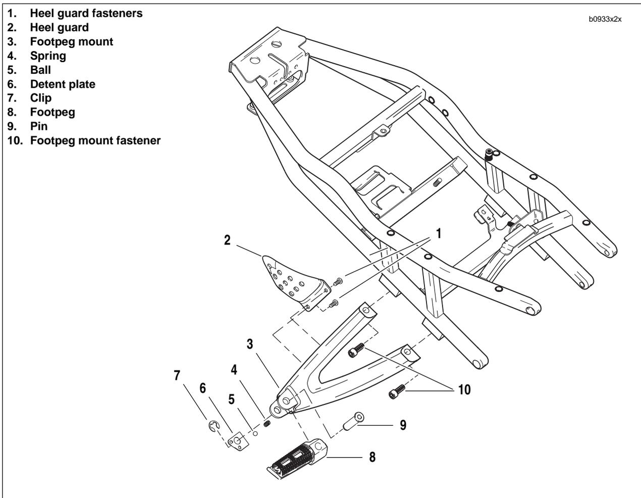
Figure 2-107. Passenger Footpeg, Mount and Heel Guard Assembly
