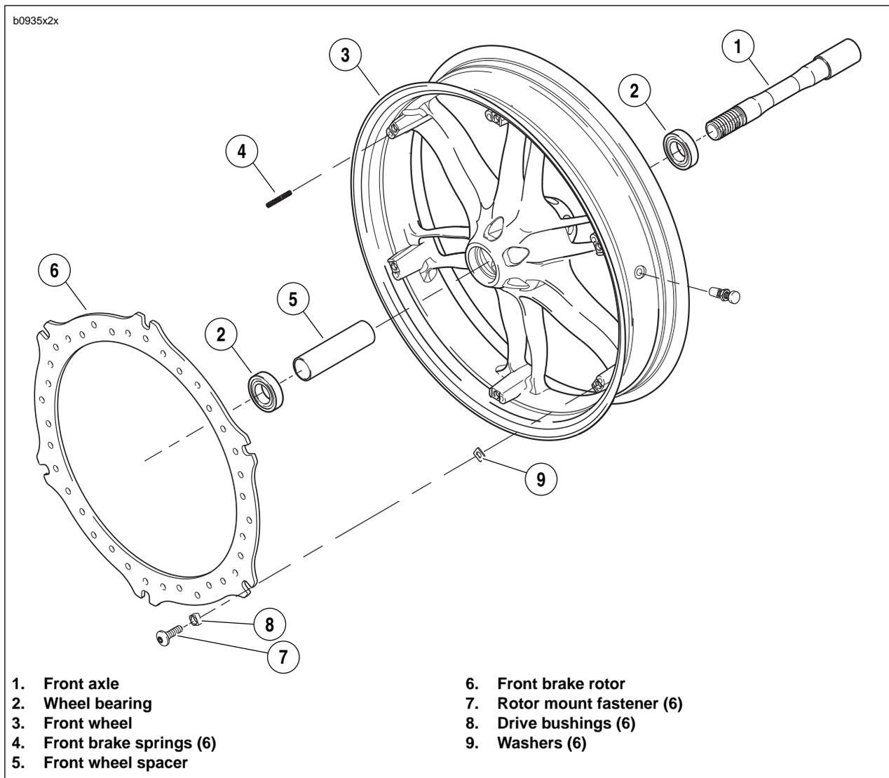
Figure 2-18. Front Wheel Assembly
