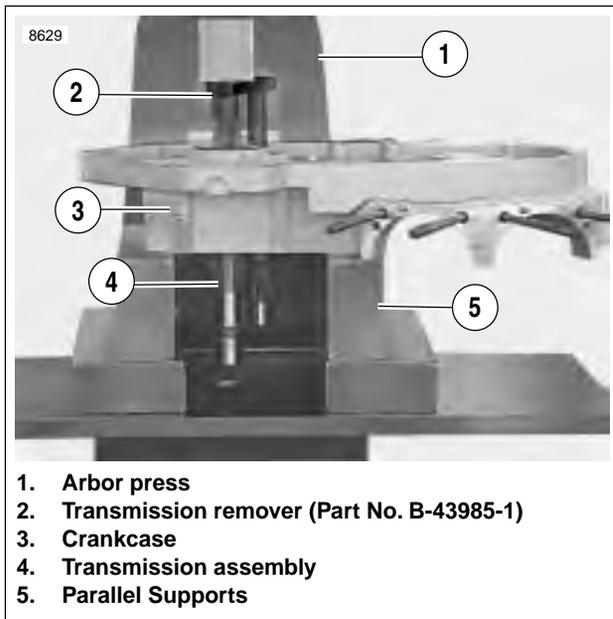
Figure 6-60. Removing Transmission Assembly from Left Case Half
