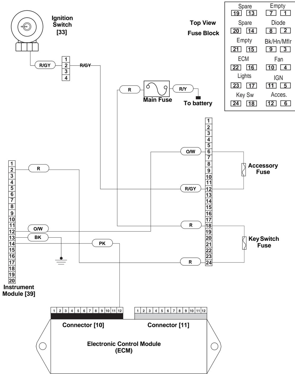
Figure 4-55. Tachometer Circuit
