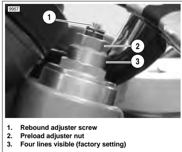
Figure 1-29. Front Fork Preload And Rebound Adjuster
