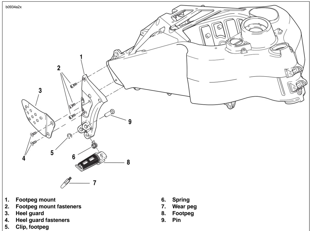
Figure 2-106. Rider Footpeg, Mount and Heel Guard Assembly
