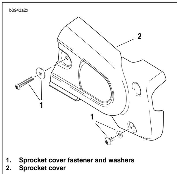
Figure 6-39. Sprocket Cover
