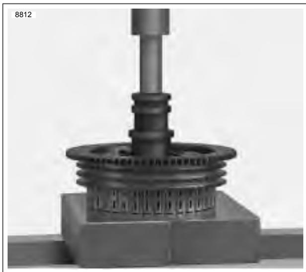
Figure 6-29. Removing Clutch Shell Needle Bearing
