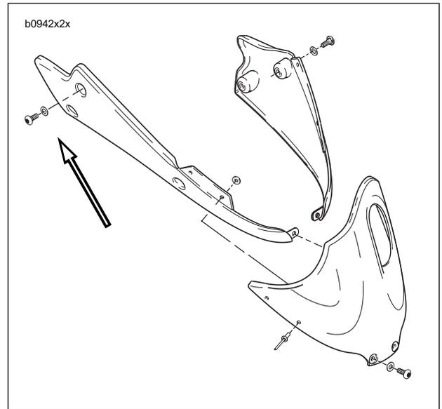
**Figure 2-108. Chin Fairing Assembly, Right Rear Fasteners**
