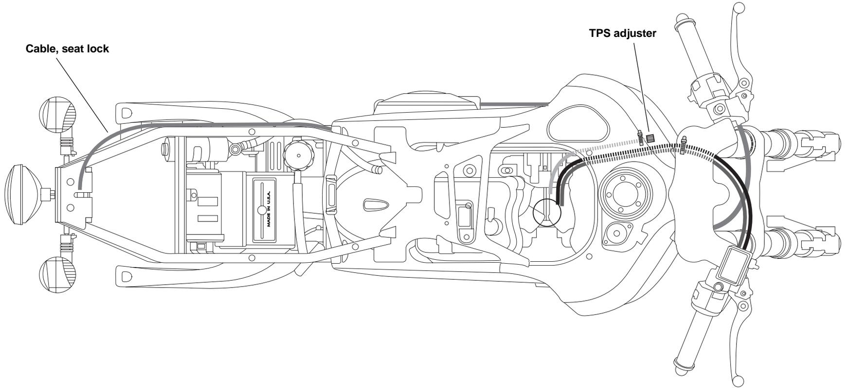
Figure D-13. Clutch, Throttle and Seat Release Cables, Top View
