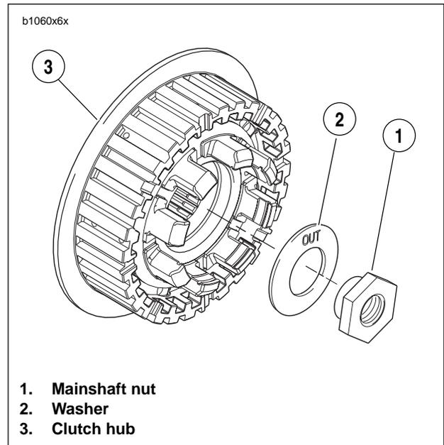
Figure 6-34. Mainshaft Nut and Washer
