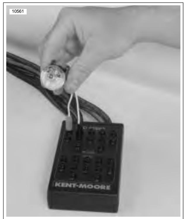
Figure 4-49. Testing Ignition Coil Connectors
