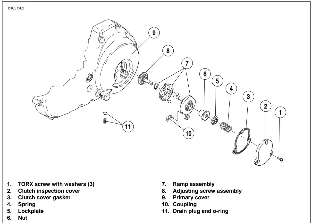
Figure 6-8. Clutch Release Mechanism
