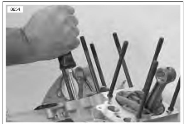
**Figure 3-130. Checking Cam Gear End Play**
