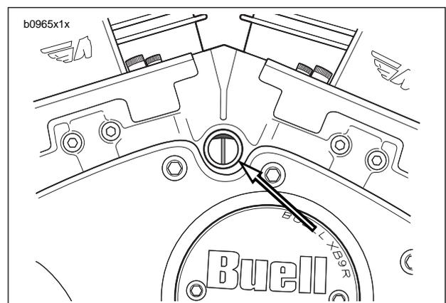
Figure 1-48. Correct Timing
