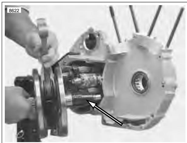
**Figure 6-86. Installing Flywheel Assembly Using Crankshaft Guide Tool (Part No. HD-42326)**
