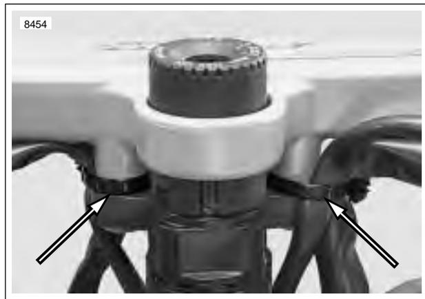
Figure 7-3. Cable Straps On Upper Fork Clamp
