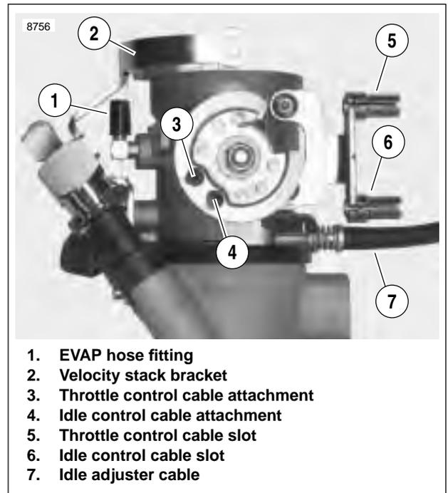
Figure 4-69. Throttle Cable Bracket (typical)
