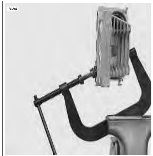
**Figure 3-82. Valve Spring Compressor (Part No. HD-34736B)**
