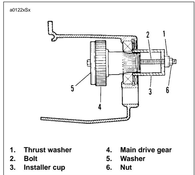
**Figure 6-73. Main Drive Gear Installation**
