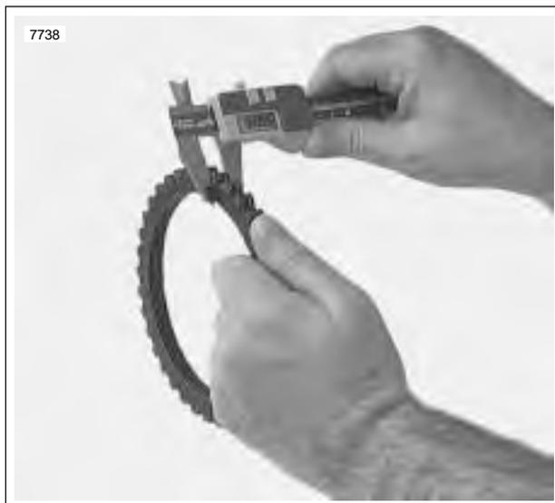
Figure 6-16. Measuring Friction Plates
