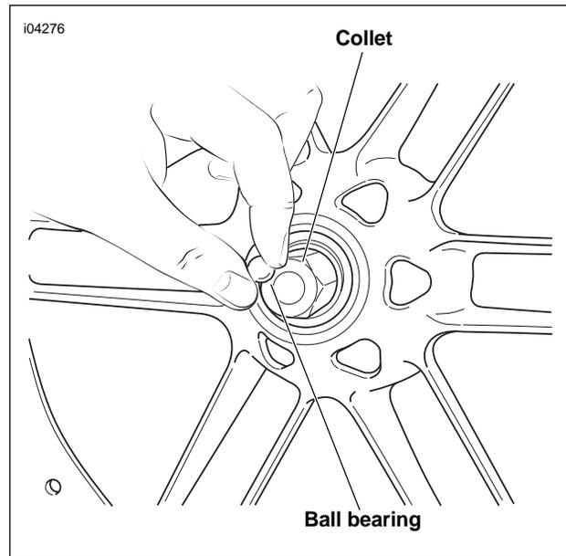
**Figure 2-8. Install Collet and Ball Bearing**
