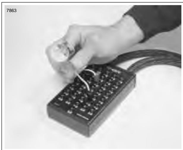
Figure 4-20. Ignition Coil Circuit Test
