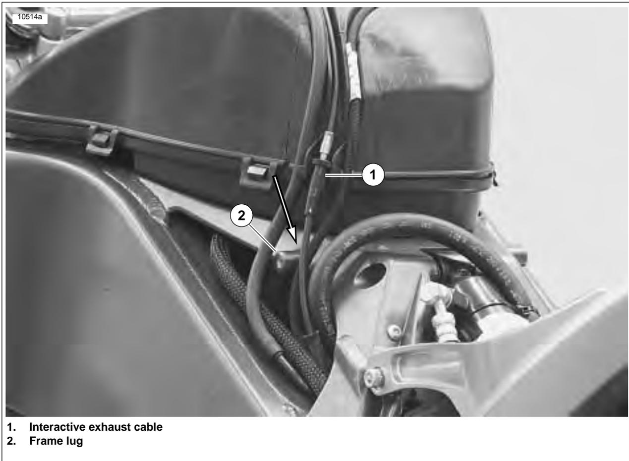
Figure 1-46. Correct Cable Routing Behind Frame Lug
