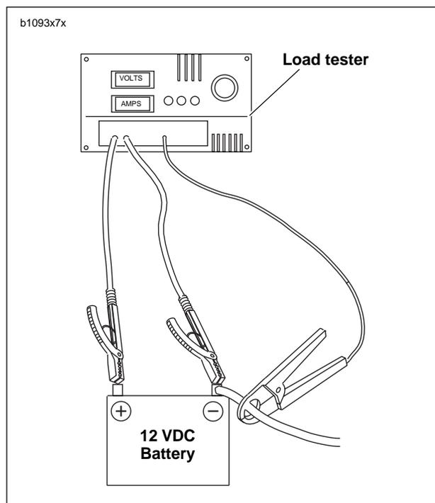
Figure 7-27. Check Current Draw (Ignition Switch On)
