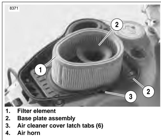
Figure 1-40. Installed Air Cleaner Filter Element
