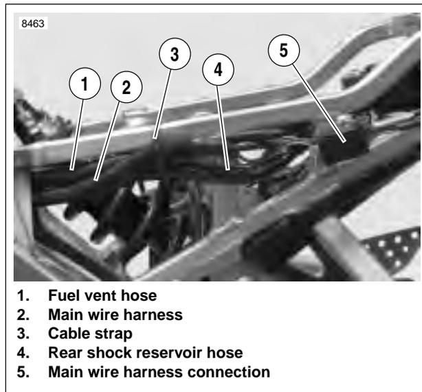
**Figure 2-116. Left Side Subframe Tail Assembly Hose and Wire Routing**
