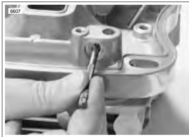
**Figure 3-69. Measuring Rocker Arm Shaft Bore Diameter in Lower Rocker Cover**
