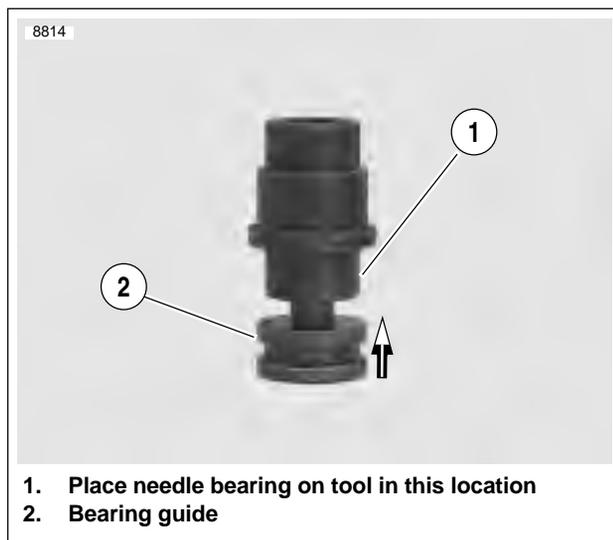
1. Place needle bearing on tool in this location
