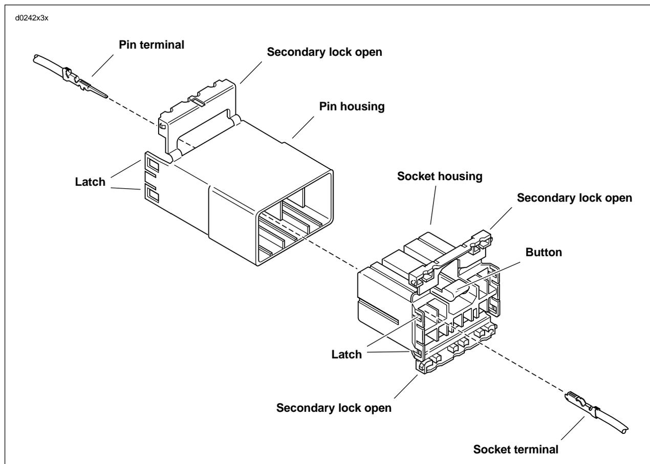
Figure B-1. 10-Place Amp Multilock Connector
