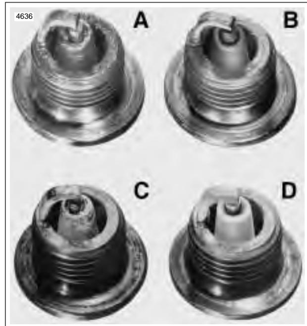
Figure 1-36. Typical Spark Plug Deposits
