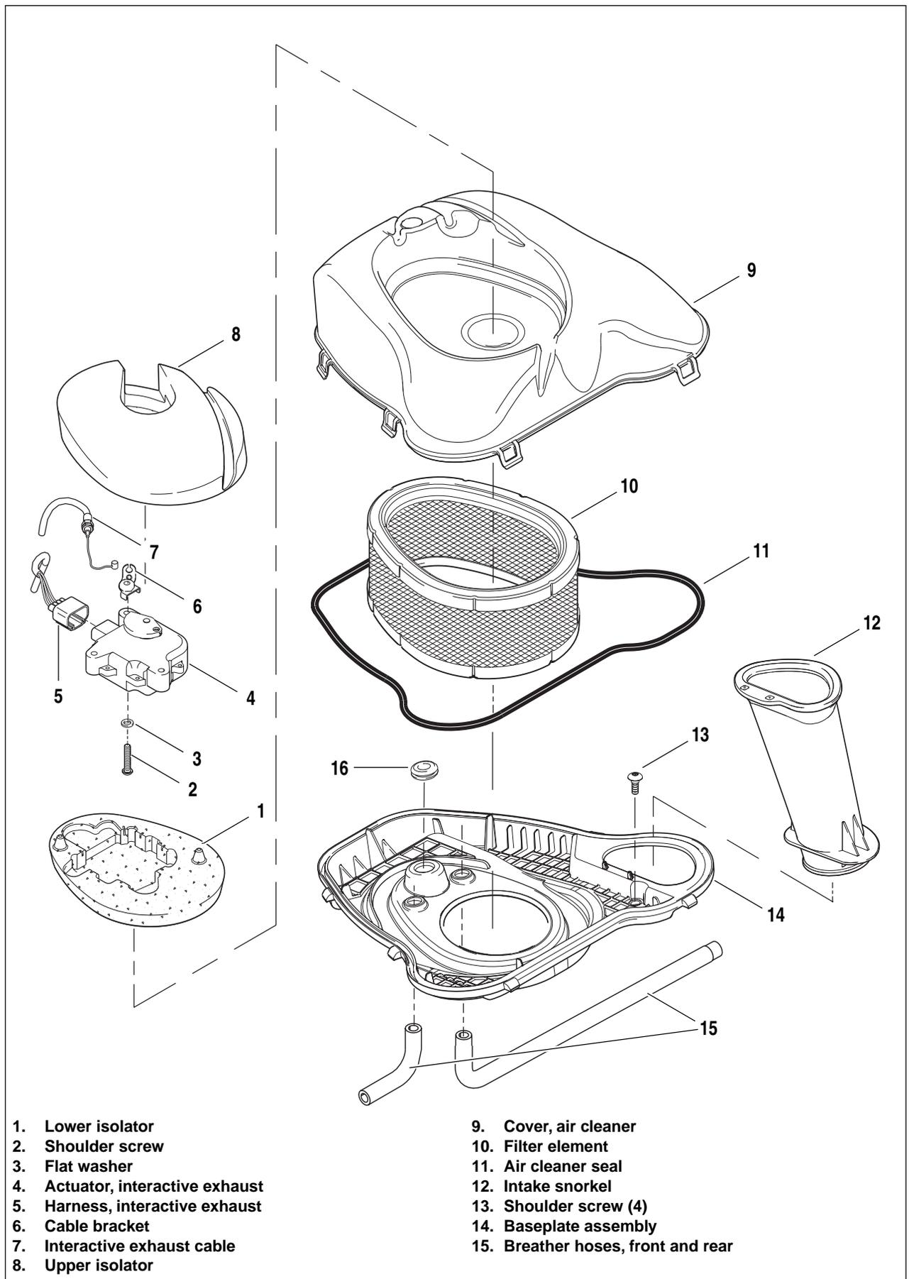
Figure 4-80. Air Cleaner Assembly (XB12) with Interactive Exhaust Components
