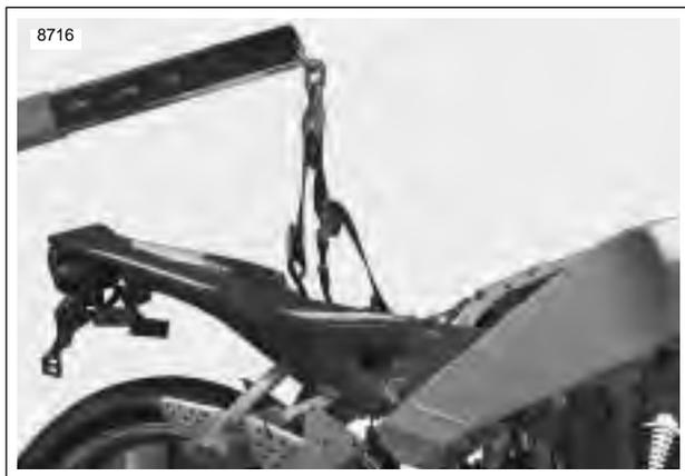
**Figure 3-24. Supporting Vehicle for Disassembly**
