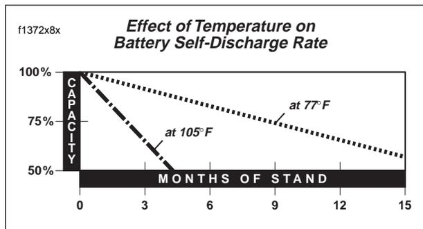
Figure 7-45. Battery Self-Discharge Rate
