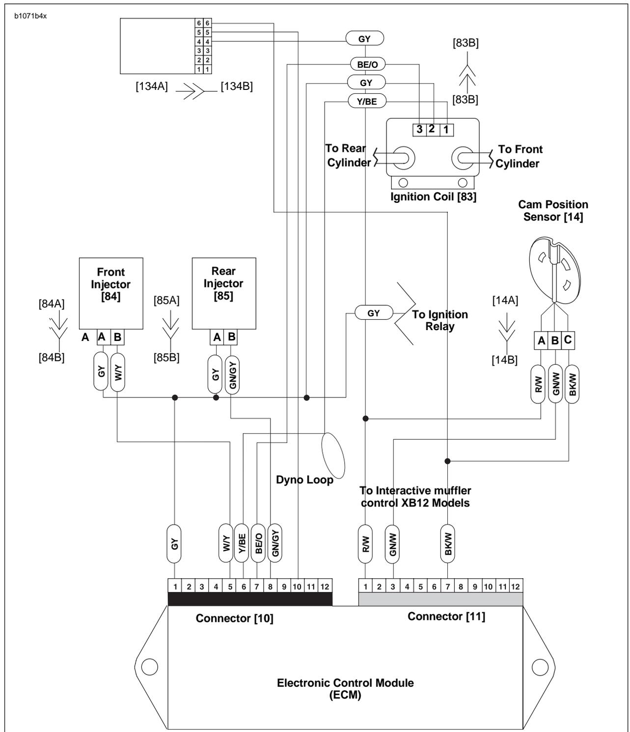
Figure 4-21. Ignition Circuit
