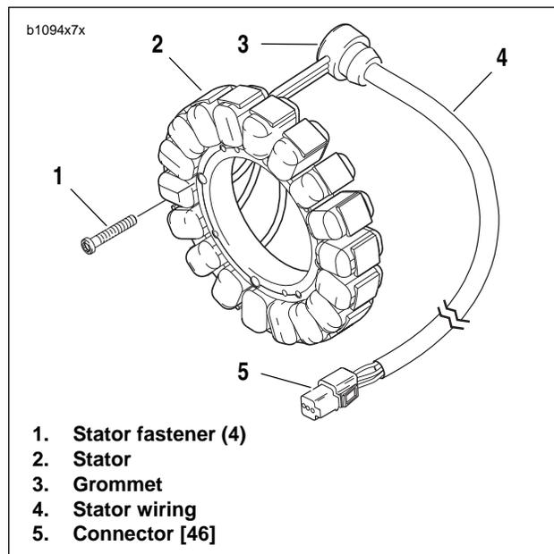
Figure 7-34. Stator Assembly
