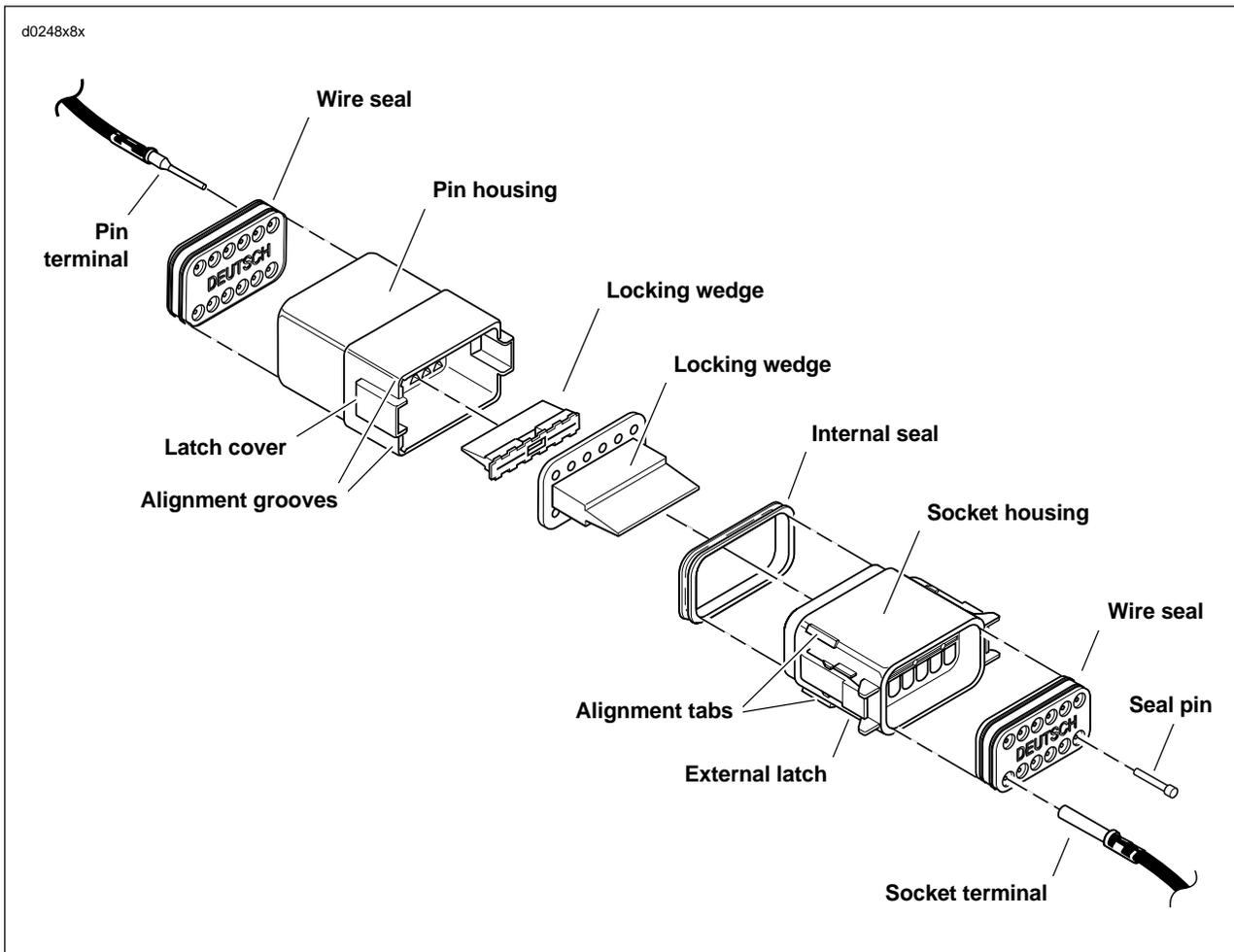
Figure B-8. 12-pin Deutsch Connector (Exploded View)
