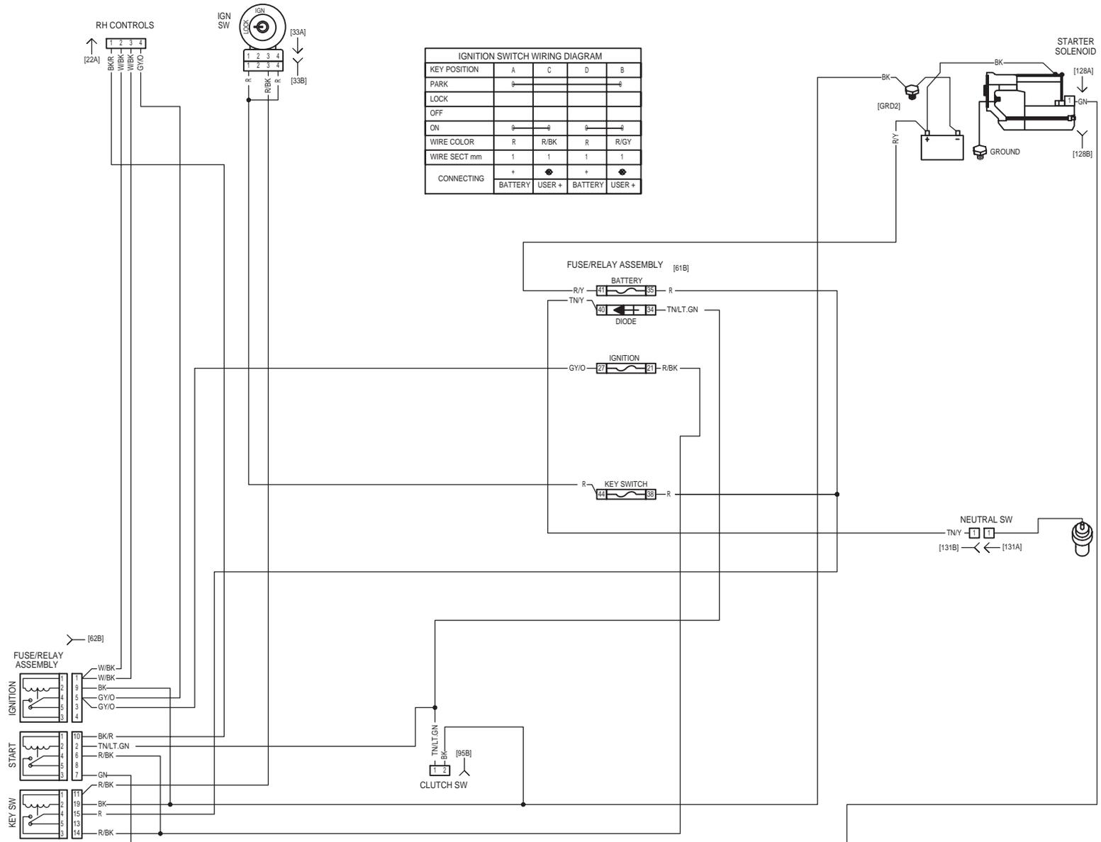
Figure 5-4. Electric Starting System Circuit
