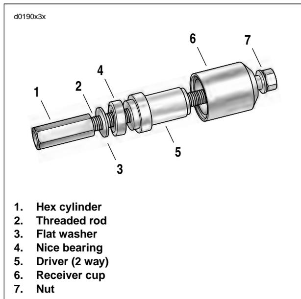
**Figure 3-101. Connecting Rod Bushing Remover/Installer (Part No. HD-95970-32D)**
