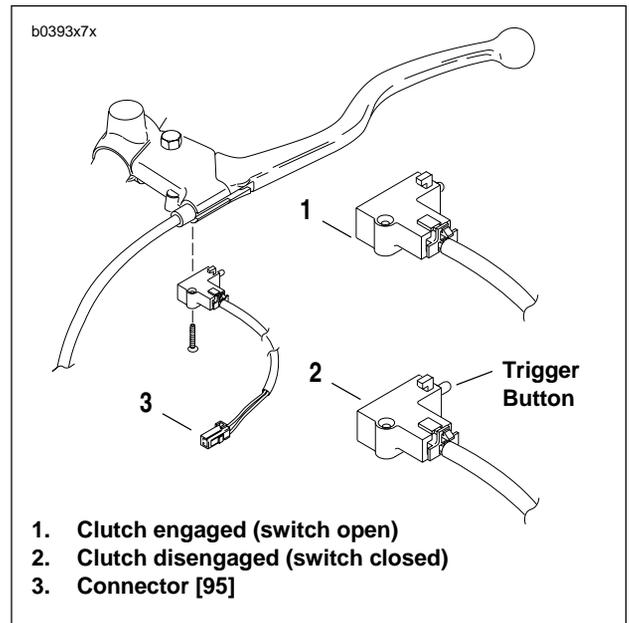
Figure 7-14. Clutch Switch
