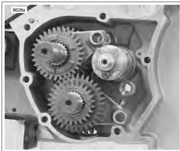
Figure 6-57. Transmission Assembly
