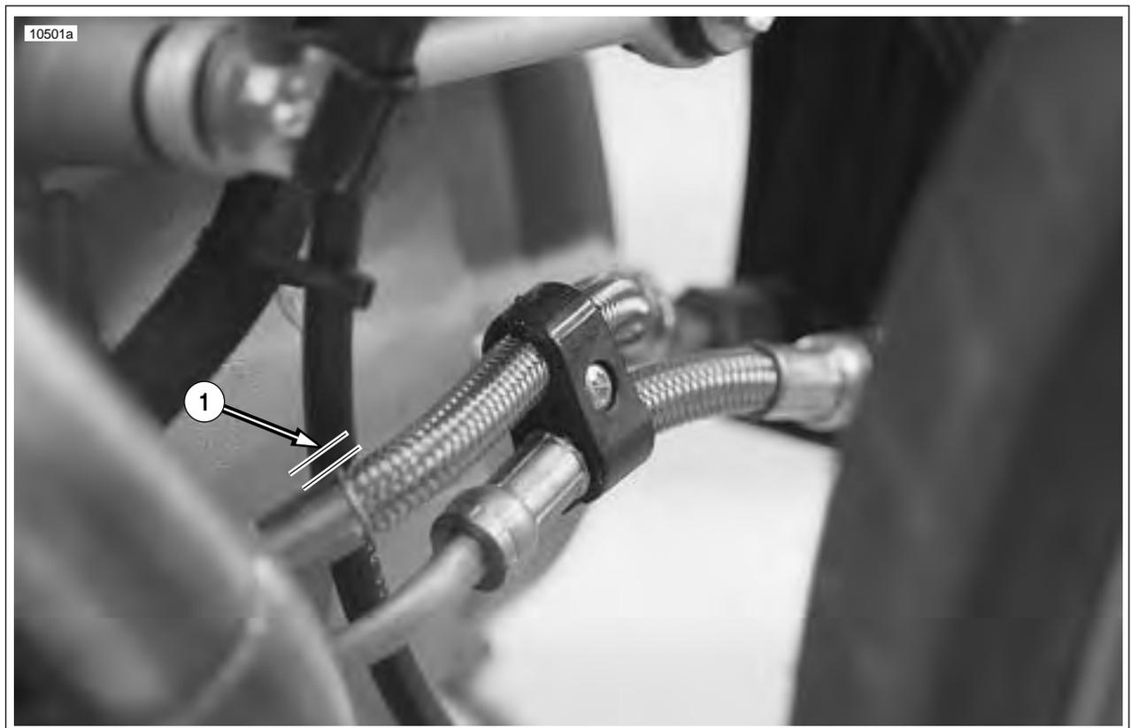
**Figure 3-12. Oil Cooler Feed and Return Oil Line 1/8-1/4 in. (3.175-6.35 mm) Clearance**
