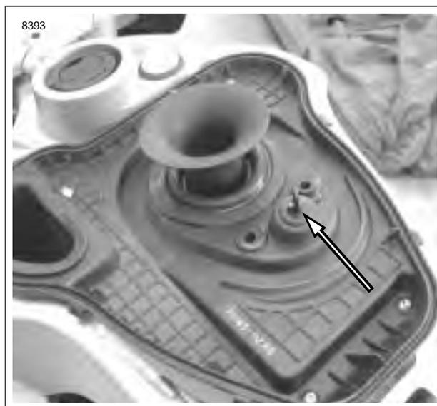
**Figure 4-46. Intake Air Temperature Sensor Installed**
