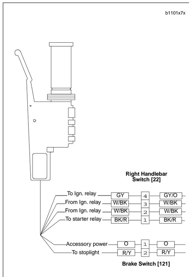
Figure 7-55. Right Handlebar Switch Connection
