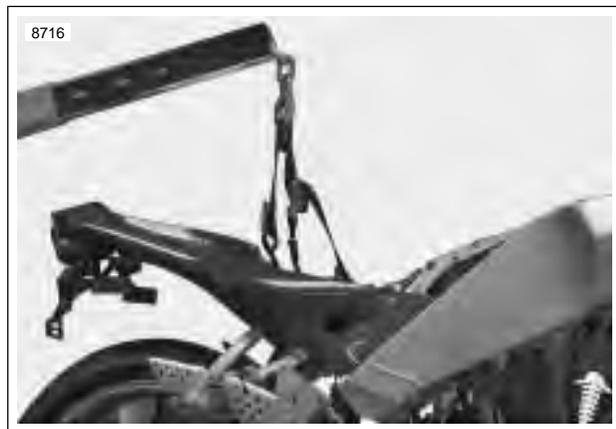
**Figure 3-41. Supporting Vehicle for Assembly**
