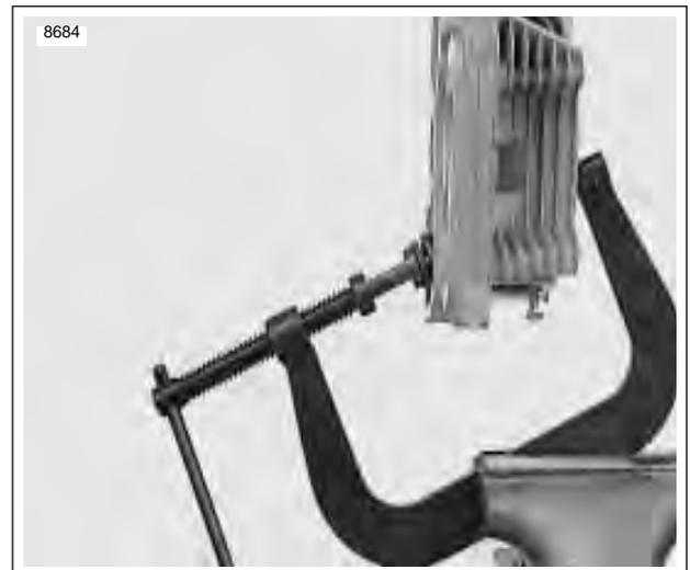
Figure 3-64. Valve Spring Compressor
