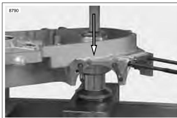
**Figure 3-139. Direction of Bearing Removal From Left Crankcase**
