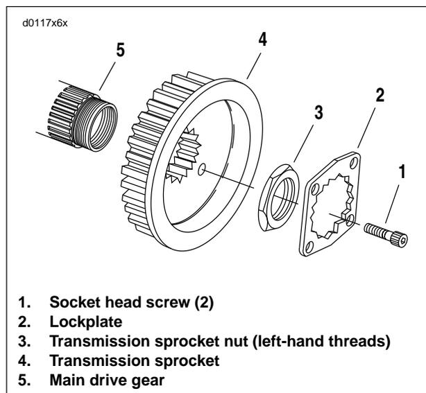
Figure 6-95. Transmission Sprocket
