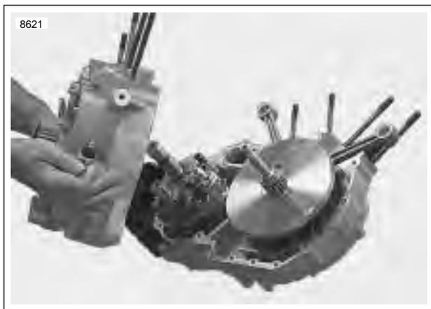
Figure 6-54. Separating Crankcase Halves
