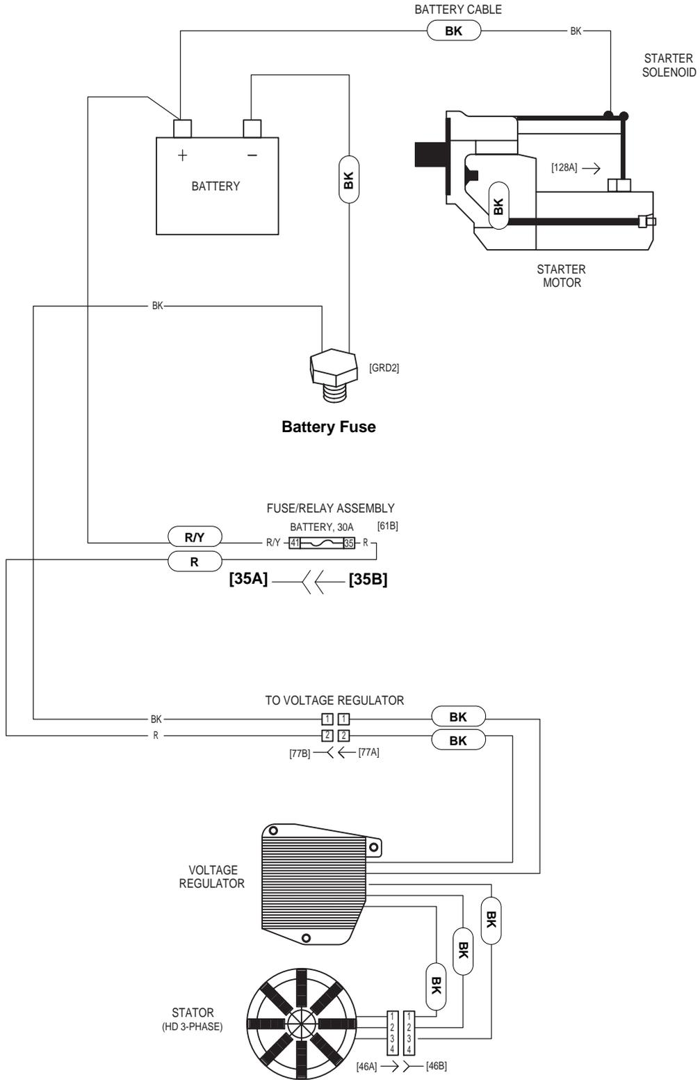
Figure 7-25. Charging System Circuit
