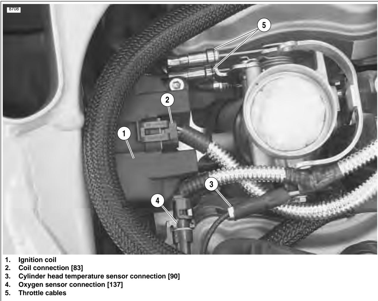
Figure 3-17. Electrical Connections and Throttle Cables (Typical)
