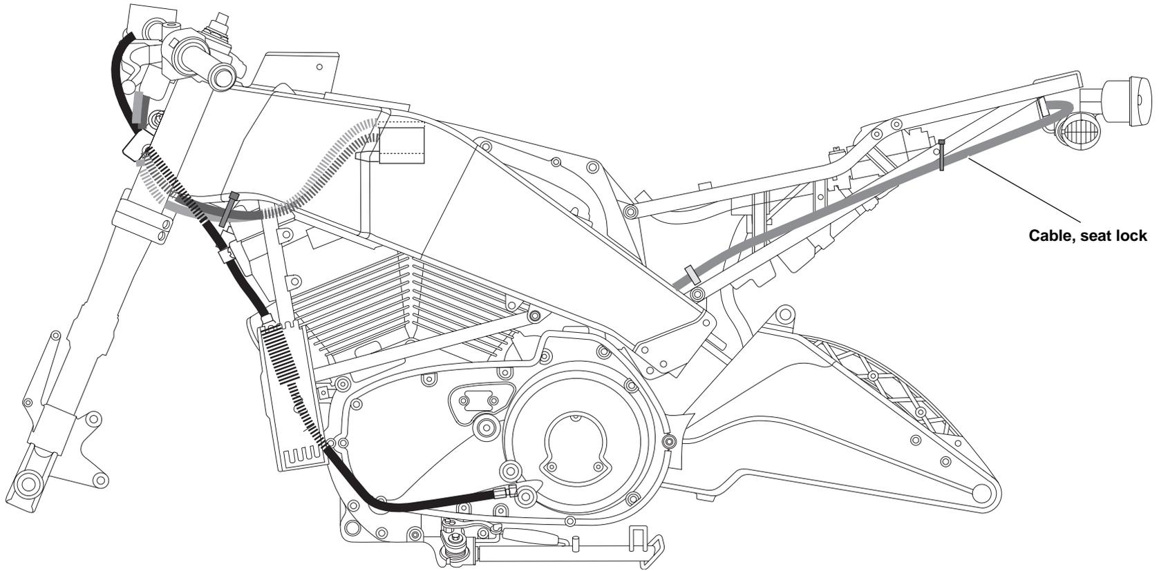
**Figure D-12. Clutch, Throttle and Seat Release Cables, Left Side View**
