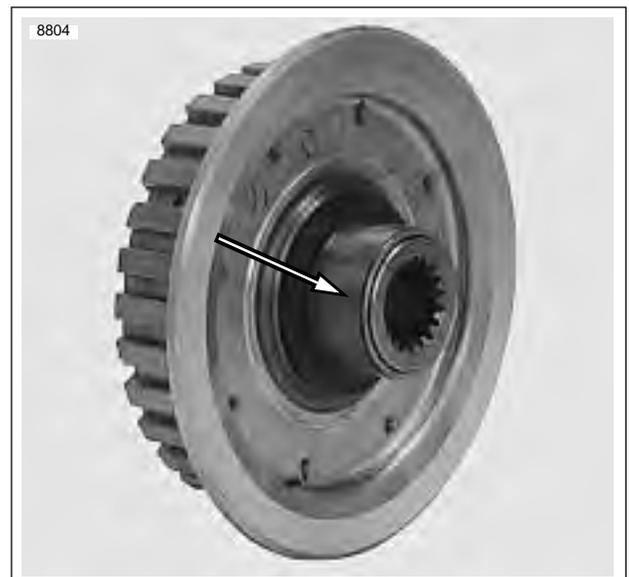
Figure 6-27. Clutch Hub Bearing Race
