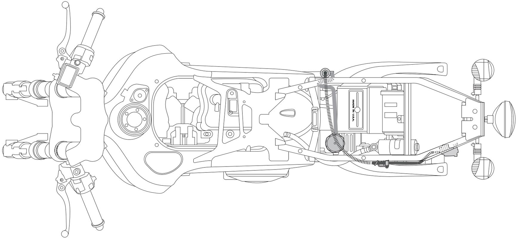
Figure D-2. Rear Brake Systems, Top View
