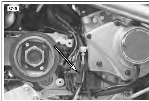
Figure 4-33. Cam Position Sensor Connector [14] (stator connector disconnected)
