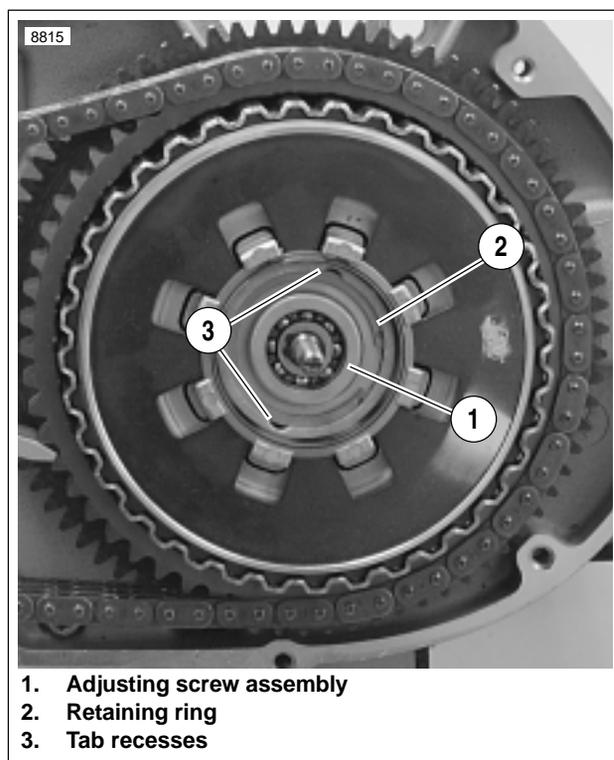
Figure 6-22. Clutch Adjusting Screw Assembly and Retaining Ring
