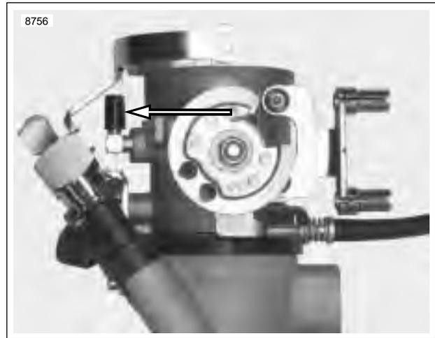
Figure 4-85. Emissions Hose Attachment, California Models Only
