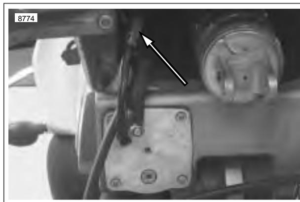
Figure 4-66. Fuel Pump connector [86] (swingarm removed for illustration)
