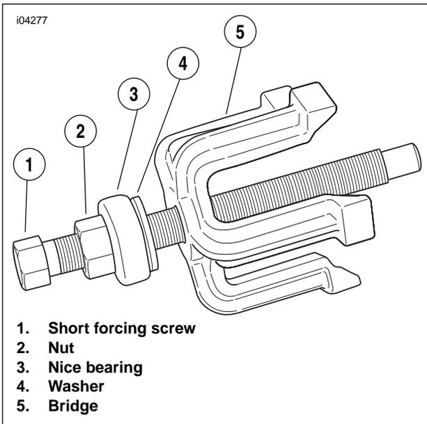
**Figure 2-7. Assemble Puller**
