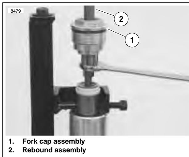
**Figure 2-71. Rebound Assembly and Fork Cap Assembly**
