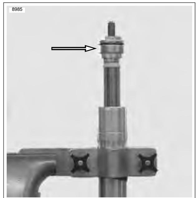
**Figure 2-66. Removing Fork Cap From Outer Tube**
